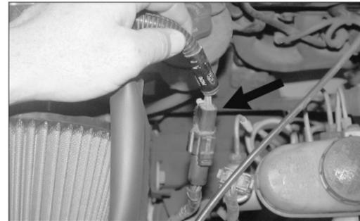
25. Reconnect the secondary mass air electrical connection as shown.
