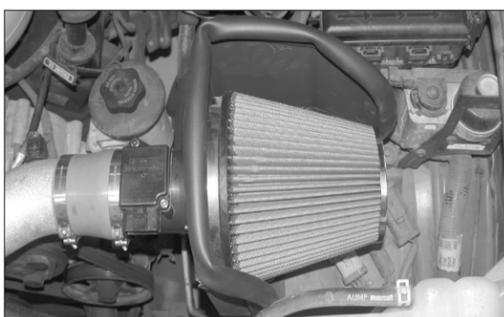
24. Install the K&N air filter and secure with the provided hose clamp as shown.
