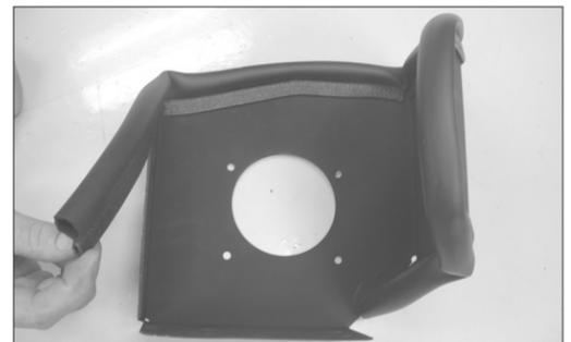
12. Install the provided edge trim onto the provided heat shield and trim to fit if necessary.
