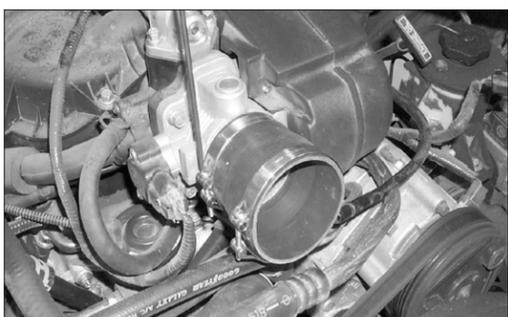
16. Install the silicone hose and hose clamps onto the throttle body and tighten as shown.
