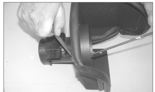
13. Assemble the provided mass air adapter, gaskets, heat shield and the stock mass air sensor using the provided hardware as shown.
