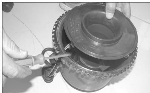
9. Using a flat blade screwdriver release the housing cover by depressing the four release clips as shown.
