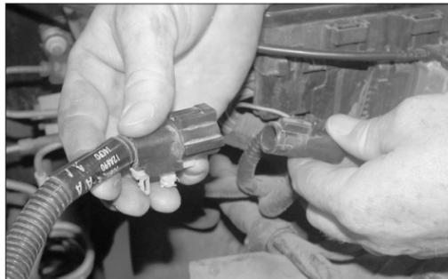
7. Disconnect the secondary mass air sensor electrical connection as shown.
