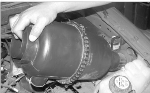
5. Pull up on the air cleaner assembly to release it from the stock grommets.
