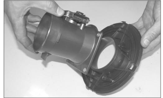
11. Remove the mass air sensor from the housing cover which is secured by two bolts.
