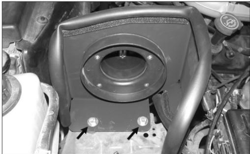
14. Secure the heat shield assembly to the stock air cleaner mounting grommets using the provided hardware as shown.
