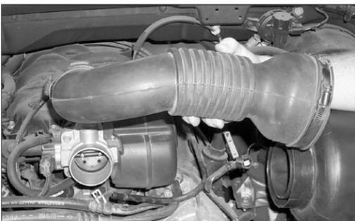
4. Loosen the hose clamps at the throttle body and at the air cleaner, then, remove the stock intake tube as shown.
