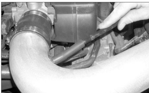
22. Reconnect the crank case vent hard line to the silicone hose on the K&N intake tube as shown. Trim to fit if necessary.
