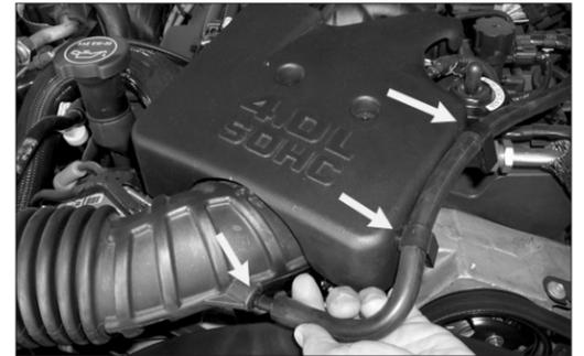
5. On vehicles that come with a second vent line, remove hose from intake tube then release the two clips that retain the hose to the engine cover.
