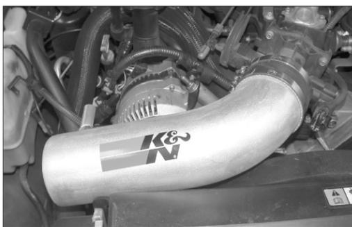
17. Re-install the K&N® intake tube onto the throttle body and mounting bracket and then secure with the provided hose clamp and hardware.
