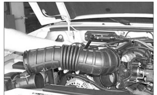
6. Loosen the hose clamp at the throttle body and at the mass air sensor, then remove the stock air intake tube as shown.
