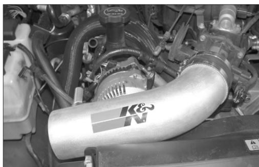
15. Install the K&N® intake tube onto the throttle body and line it up with the tube-mounting bracket, then secure with the hose clamp and hardware provided.
