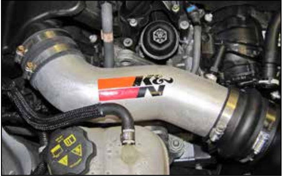
17. Install the K&N® intake tube into the coupler at the intake plenum and then slide the hump coupler onto the filter adapter. Adjust the intake tube for best fit and then secure with the provided hose clamps and heat shield mounting hardware.
