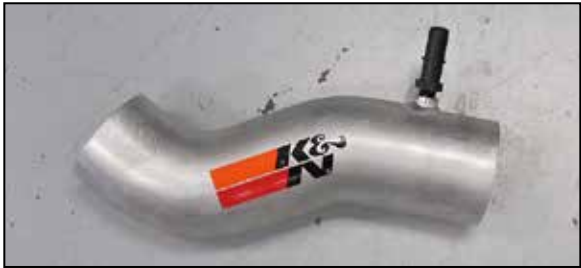
15. Install the provided quick disconnect fitting into the K&N® intake tube as shown. NOTE: Plastic NPT fittings are easy to cross thread. Install the vent fitting "hand" tight, then turn it two complete turns with a wrench.
