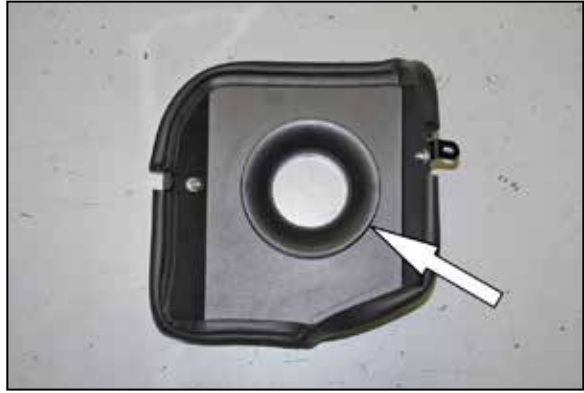
11. Install the filter adapter into the heat shield and secure with the provided hardware.
