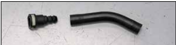
19. Remove the quick disconnect fitting from the factory flexible crank case vent line.
