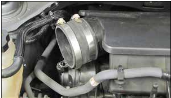
14. Install the provided coupler hose (08690) onto the intake plenum and secure with the provided hose clamp.
