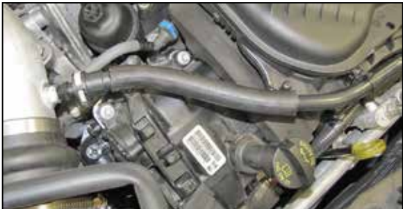
20. Install the factory quick disconnect fitting into the provided crank case vent hose and then install the assembly onto the factory hardline and connect the quick disconnect fitting to the fitting installed into the K&N® intake tube.
