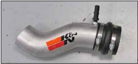
16. Install the provided hump coupler (5-576) all the way onto the K&N® intake tube but do not secure at this time.
