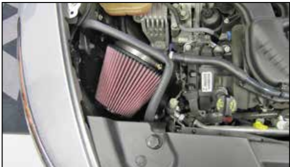
13. Install the heat shield assembly into the vehicle and secure with the hardware removed in step #6. NOTE: Do not completely tighten at this time.
