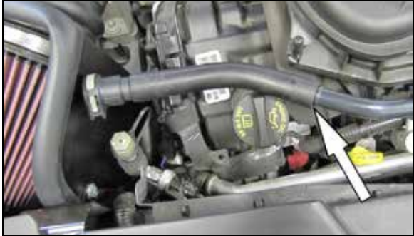
18. Remove the flexible crank case vent line from the hard line.
