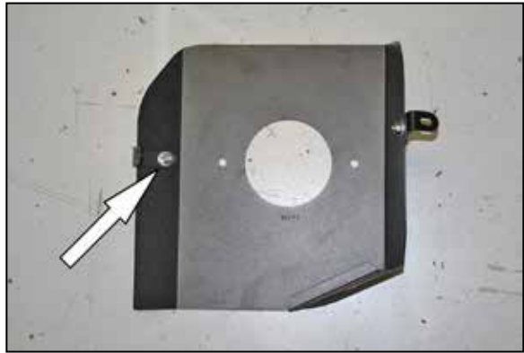
8. Install the heat shield mounting bracket (070712) onto the heat shield as shown using the provided hardware.
