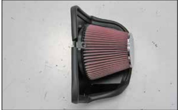
12. Install the K&N® air filter onto the filter adapter and secure with the provided hose clamp.
