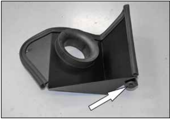
15. Install the factory mounting grommet into the heat shield as shown.
