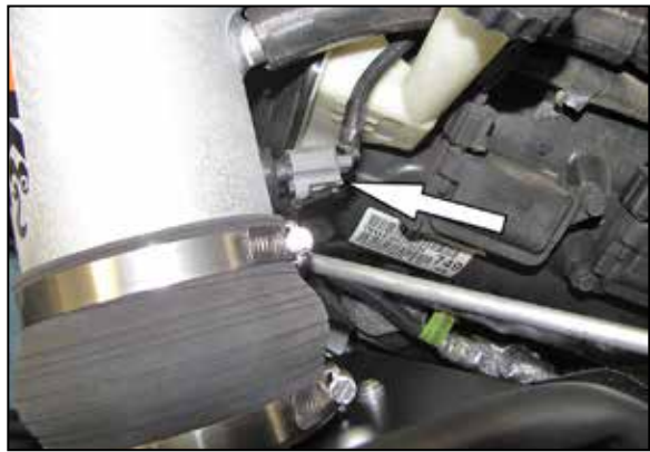
23. Reconnect the inlet air temperature sensor electrical connection.
