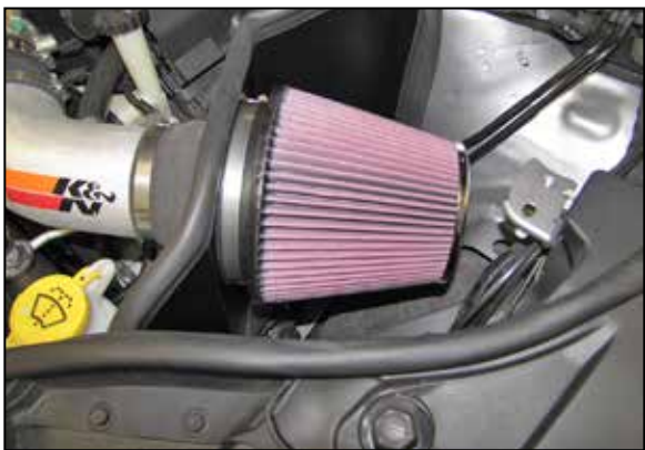
25. Install the K&N® air filter and secure with the provided hose clamp. NOTE: Drycharger® air filter wrap; part # RF-1042DK is available to purchase separately. To learn more about Drycharger® filter wraps or look up color availability please visit http://www.knfilters.com ®.
