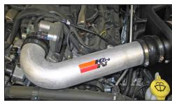
21. Install the K&N® intake tube into the hump hose at the filter adapter and then into the hose at the throttle body. Adjust the tube and heat shield for best fit and clearance and then secure with the provided hose clamps
