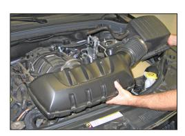
7. Remove the upper air box and intake tube assembly.
