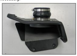
14. Install the provided silicone hump hose (084057) onto the filter adapter and secure with the provided hose clamp.
