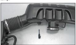
18. Release the locking tab and then remove the inlet air temperature sensor from the factory intake tube by twisting counter clockwise.
