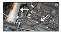
22. Install the crank case vent hose onto the 90° vent fitting and then attach the open end to the valve cover port.
