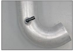
20. Install the 90° npt fitting into the K&N $^{\circ}$  intake tube as shown.
