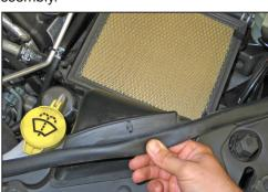
8. Unhook the sealing trim from the fresh air intake scoop.
