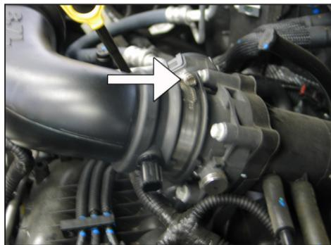
5. Loosen hose clamp at throttle body.
