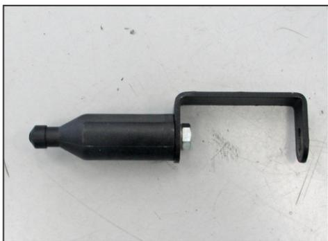
14. Install the heat shield mounting standoff onto the mounting bracket (083151) using the provided hardware as shown.
