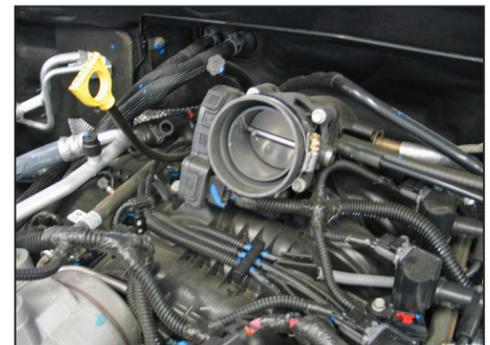
8. Install the silicone hose (084034) onto the throttle body and secure with the provided hose clamp.
