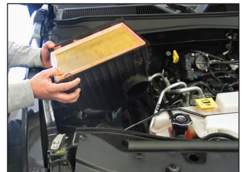
7. Lift up the lower airbox assembly to dislodge it from the mounting grommets, then disconnect the fresh air duct from the lower airbox and then remove the lower airbox from the vehicle.
