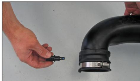
21. Remove inlet air temperature sensor from factory tube as shown.
