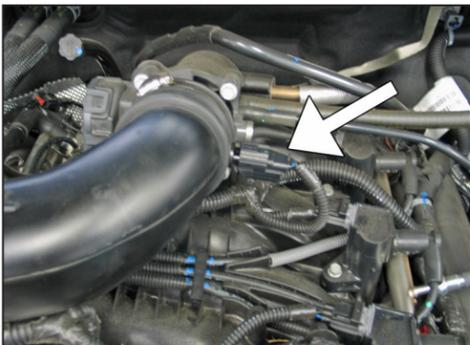
2. Release the red locking tab and then disconnect the inlet air temp sensor electrical connection.
