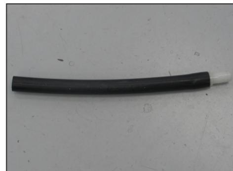
24. Install the provided hose mender into the provided crankcase vent hose as shown.
