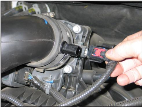
2. Release the red locking tab and then disconnect the temperature sensor electrical connection.
