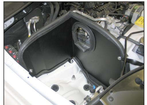
22. Install the heat shield assembly into the vehicle. Secure the rear of the heat shield to the mounting bracket installed onto the ECU. Secure the front heat shield mounting bracket to the radiator core support at the drilled location. Secure the bottom of the heat shield to the inner fender stud.
