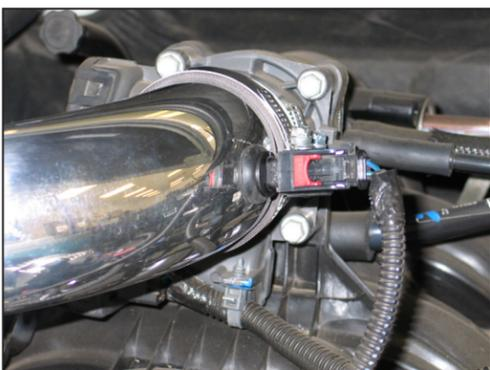
29. Reconnect the inlet air temperature sensor electrical connection.
