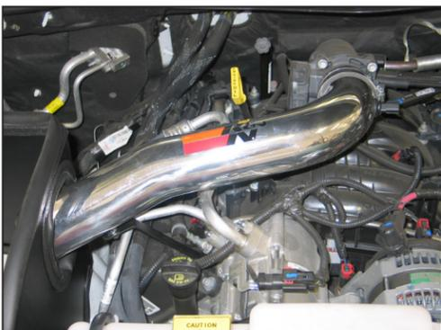
28. Install the K&N® intake tube into the silicone hose at the throttle body and align with the tube mounting bracket installed during step #11. Secure the intake tube with the provided hose clamp and hardware.
