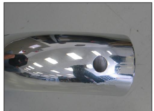
24. Remove the K&N® intake tube and drill a 3/4" id hole into the K&N® intake tube at the marked location.
