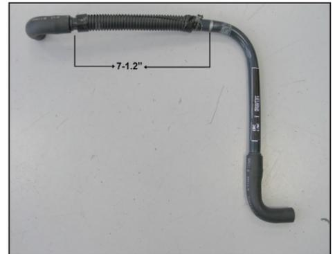
7. Using a knife, cut the crank case vent hose 7-1/2" from the valve cover elbow fitting as indicated.
