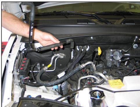
6. Remove the crank case vent tube assembly from the valve cover as shown.
