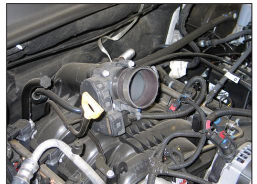
9. Install the silicone hose (084036) onto the throttle body and secure with the provided hose clamp.
