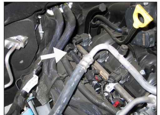
8. Reinstall the modified crank case vent tube onto the valve cover as shown.
