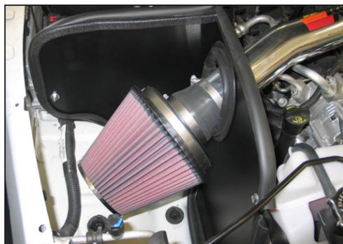
33. Install the filter assembly onto the K&N® intake tube and secure with the provided hose clamp.
