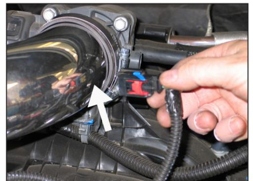
23. On vehicles equipped with an inlet air temperature sensor, install the K&N® intake tube into the silicone hose at the throttle body. Position the inlet air temperature sensor electrical connection for best fit. Mark the location for drilling.
