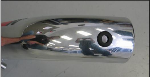
26. Install the supplied grommet into the K&N® intake tube as shown.
