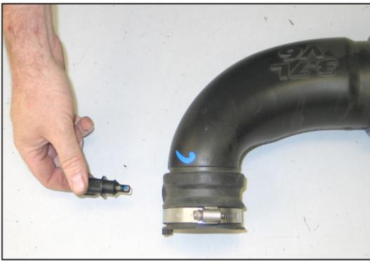
25. Remove the air temperature sensor from the factory intake tube as shown.
