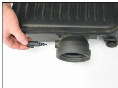
18. Twist the air temperature sensor counter clockwise and remove it from the stock intake plenum.
