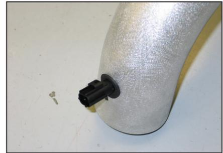
20. Install the air temperature sensor into the grommet installed into the K&N® intake tube in step #17.
