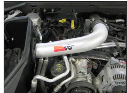
21. Install the K&N® intake tube into the silicone hose on the throttle body and position so the tube aligns with the mounting bracket. Secure the tube with the provided hose clamp and hardware.
