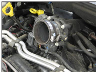
16. Install the provided silicone hose (084036) onto the throttle body and secure with the provided hose clamps.
