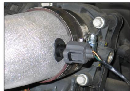
22. Reconnect the air temperature sensor electrical connection.
