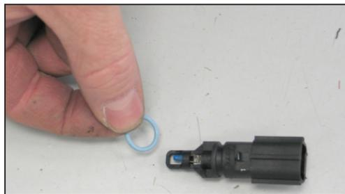
19. Remove the "O" ring from the air temperature sensor.
