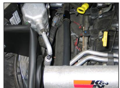
23. Install the provided silicone hose onto the fitting on the K&N® intake tube and then attach the open end onto the hose to the factory crankcase tube.
