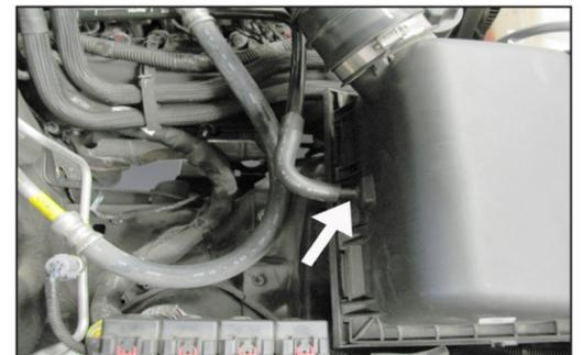
7. Disconnect the crankcase vent hose from the airbox.
