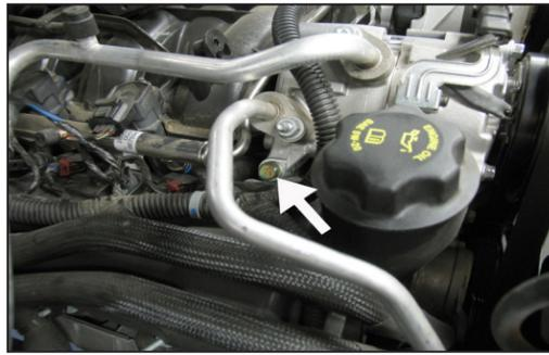
15. Remove the A/C mounting bolt shown.
