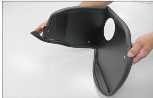
18. Install the provided edge trim onto the heat shield.
