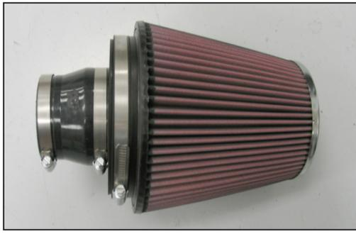
28. Install the silicone hose (08724) onto the air filter adapter and secure with the provided hose clamp.
