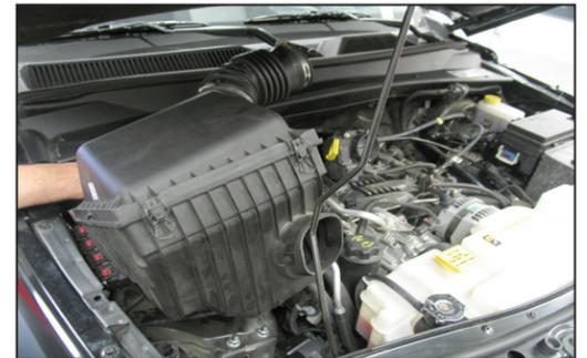
8. Pull up on the airbox assembly to dislodge it from the mounting grommets and then remove the airbox assembly from the vehicle.
