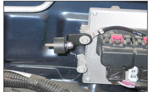
21b. On 2008 and later vehicles, attach the "L" bracket assembly from step #21a. to the ECU using the factory bolt removed in step #11a.
