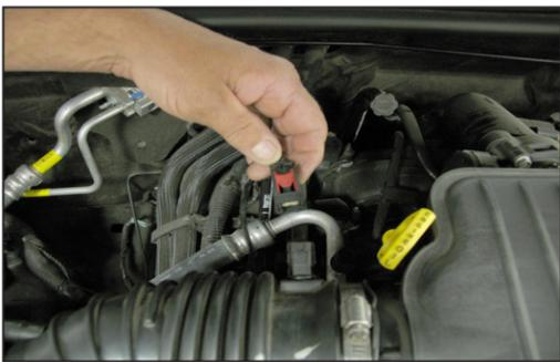
2. Release the red locking tab and then disconnect the air temperature electrical connection.
