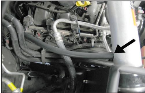
30. Install the provided silicone crankcase vent hose onto the fitting on the engine and then connect to the fitting on the K&N® intake tube. **NOTE: Some trimming of the hose may be necessary.**
