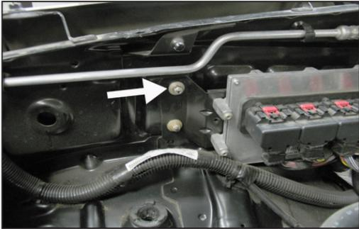
11. On 2007 model year vehicles, remove the front-upper ECU mounting nut shown.
