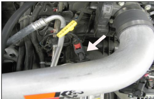
31. Reconnect the air temperature sensor electrical connection.
