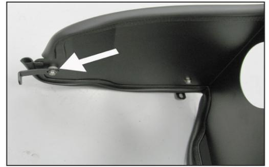
21. On 2007 and later vehicles, install the remaining small "L" bracket (06464) onto the heat shield with the provided spacer and hardware.
