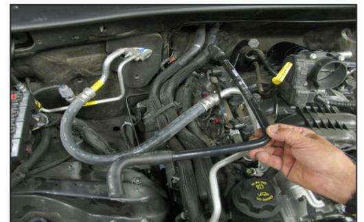
9. Unhook the crankcase vent hose from fitting on the valve cover and then remove the crankcase vent hose assembly from the vehicle.
