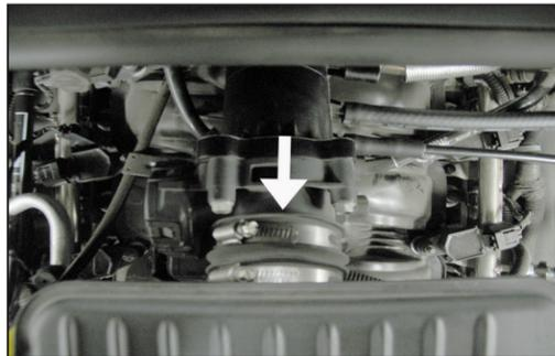
5. Loosen the hose clamp that secures the intake plenum to the throttle body.
