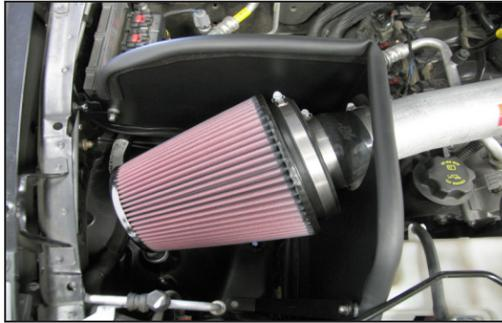
29. Install the filter assembly onto the K&N® intake tube and secure with the provided hose clamp.
