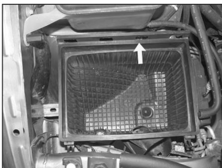
13. Remove the air box mounting bolt shown.
