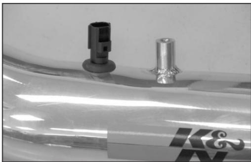
28. Install the air temperature sensor into the grommet installed into the K&N® intake tube in step #25.
