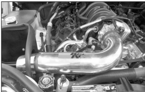
29. Install the K&N® intake tube into the silicone hose at the throttle body and onto the tube mounting bracket, then secure with the provided hose clamp and hardware.
