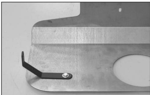
15. Install the supplied "C" bracket (07171) onto the heat shield as shown with the provided hardware. **NOTE: Due to manufacturing tolerances, it may be necessary to use the provided spacer and longer bolt to attach the mounting bracket to the heat shield. This will enable the mounting bracket to align with the longer air box mounting brackets on some vehicles.**
