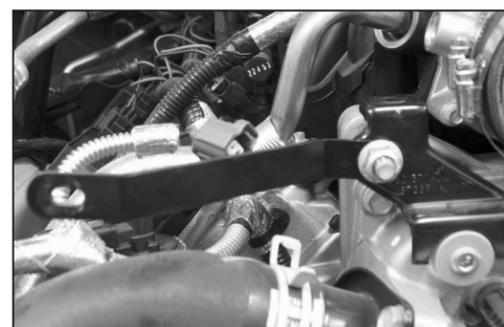
24. Install the tube mounting bracket onto the plenum mount and secure with the factory nut removed in step #23.
