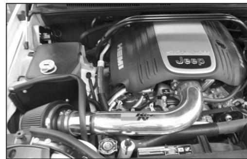
36. Reinstall the engine cover and oil filler cap. Reconnect the vehicle's negative battery cable. Double check to make sure everything is tight and properly positioned before starting the vehicle.
