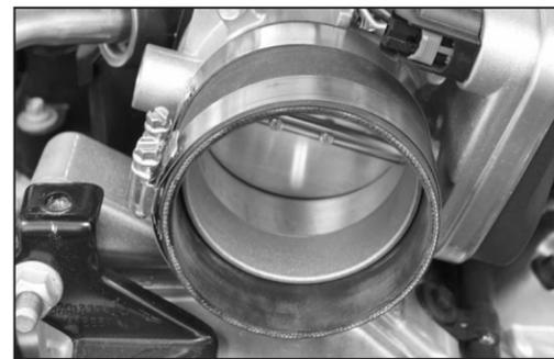
22. Install the silicone hose (08630) onto the throttle body and secure with the hose clamp provided.
