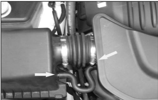
2. Loosen the hose clamp, which secures the stock intake tube to the intake plenum, and disconnect the crank case vent hose from the air box lid.
