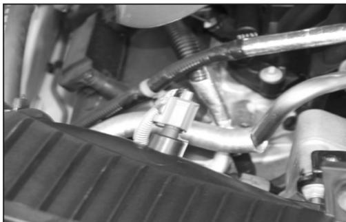
6. Disconnect the air temperature sensor electrical connection and then remove the intake plenum from the vehicle.
