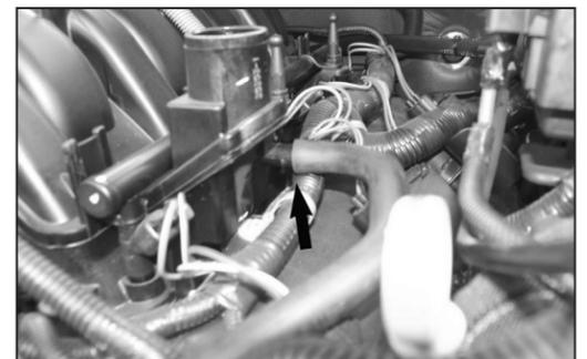
8. Remove the crank case vent hose from the valve cover.
