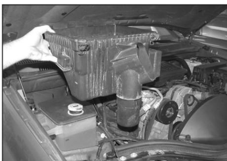
14. Lift the lower air box and remove it from the vehicle as shown.
