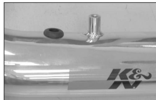
25. Install the provided grommet into the K&N® intake tube as shown.
