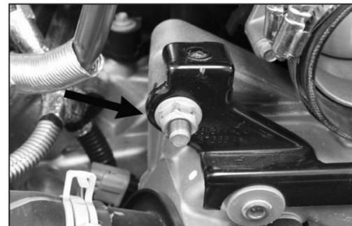
23. Remove the intake plenum mount nut shown. **NOTE: Do not discard as this nut will be reused.**
