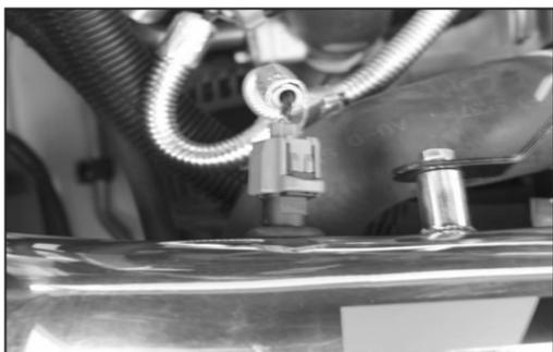
31. Reconnect the air temperature sensor electrical connection as shown.
