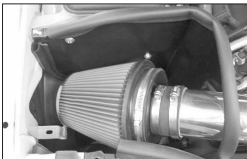
34. Install the air filter assembly onto the K&N® intake tube as shown and secure with the provided hose clamp.
