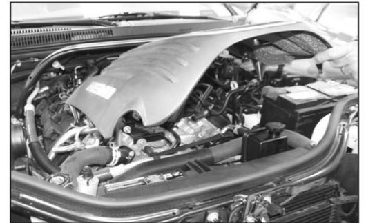
7. Remove the engine cover from the engine.
