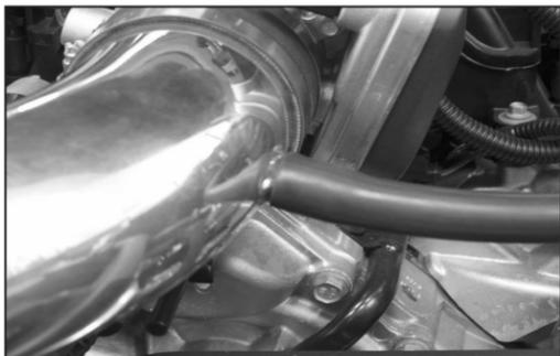
30. Install the provided crank case vent tube onto the valve cover and then onto the K&N® intake tube as shown.
