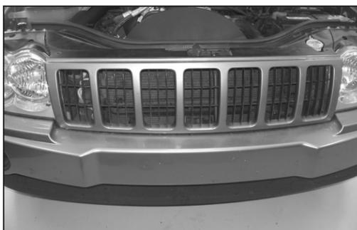
35. Reinstall the grill assembly with the factory retaining clips removed in step #5.
