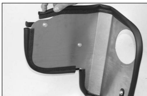
19. Install the long edge trim onto the heat shield as shown.
