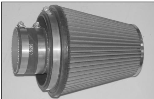
33. Install the silicone (08630) onto the air filter assembly and secure with the provided hose clamp.
