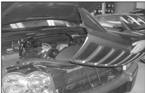
11. Remove the six grill retaining clips from the grill, then tilt the grill forward and lift to remove from the vehicle.
