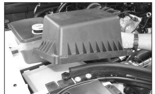
9. Unhook the air box lid retaining clamps and then remove air box lid and filter.
