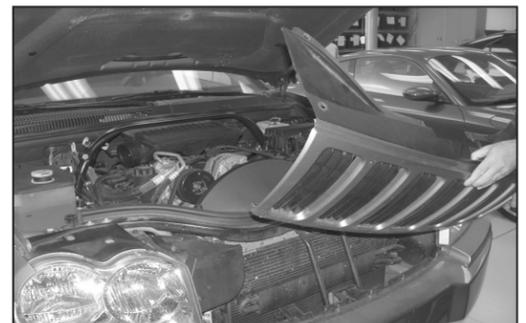
6. Remove the six grill retaining clips from the grill, then tilt the grill forward and lift to remove from the vehicle.
