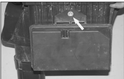
14. Remove the bolt that secures the vacuum reservoir to the airbox and then remove the reservoir from the airbox.
