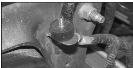
18. Install the 6mm male/male rubber mounted stud onto the upper airbox mount as shown.
