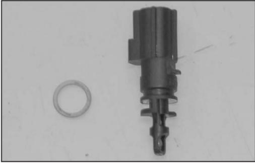
26. Remove the rubber sealing "O" ring from the air temperature sensor as shown.
