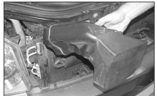
7. Pull the fresh air duct forward to disconnect it from the airbox and then remove it from the vehicle.
