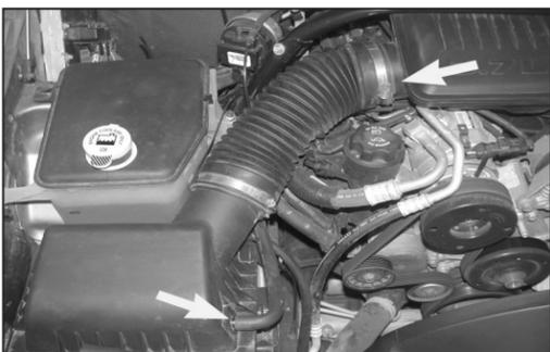
2a. Loosen the hose clamp, which secures the stock intake tube to the intake plenum, and disconnect the crankcase vent hose from the air box lid.
