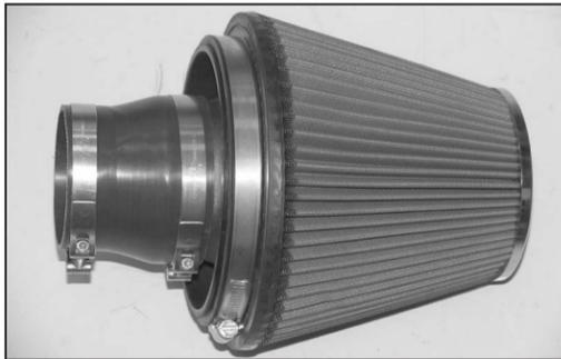
33. Install the silicone hose (084055) onto the air filter assembly and secure with the provided hose clamp.
