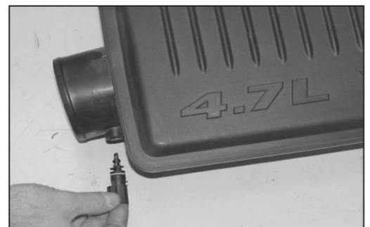
24. Rotate the air temperature sensor counter clockwise and remove the sensor from the stock intake plenum as shown.
