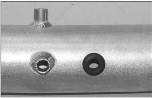
25. Install the supplied rubber grommet into the K&N® intake tube as shown.
