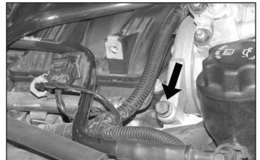
22. Remove the lower rear A/C mounting bolt shown. **NOTE: This bolt will be reused.**
