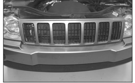
35. Reinstall the grill assembly with the factory retaining clips removed in step #5.
