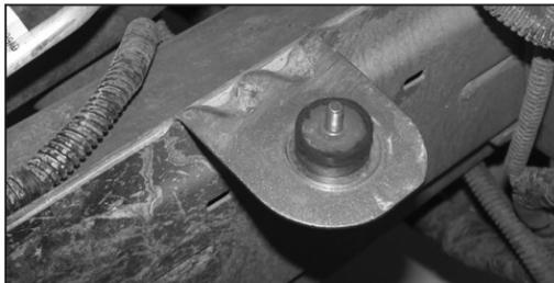
17. Using the two fender washers and one rubber washer, install the 6mm male/female rubber mounted stud onto the lower airbox mount as shown.
