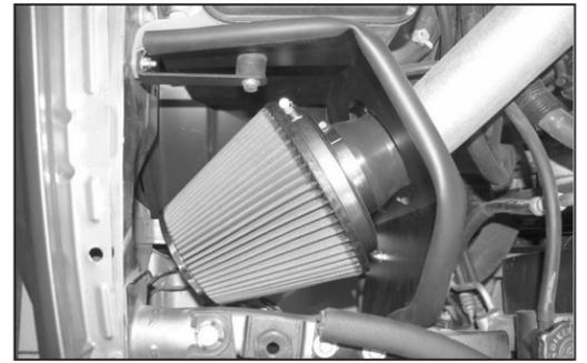
34. Install the air filter assembly onto the K&N® intake tube as shown and secure with the provided hose clamp.
