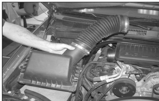
3. Unclip the upper airbox retaining clips and remove the upper airbox and intake tube assembly as shown.
