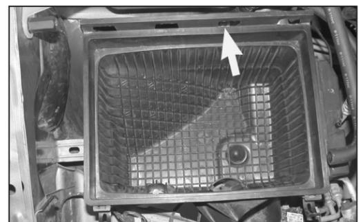
8. Remove the airbox mounting bolt shown.
