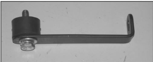
11. Install the 1/4"-20 male/female rubber mounted stud onto the "L" bracket (070952) with the provided hardware as shown.
