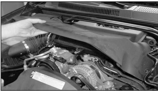
2. On 2008 and later model vehicles, pull up on the engine cover to dislodge it from the mounting grommets and then remove the engine cover from the vehicle.
