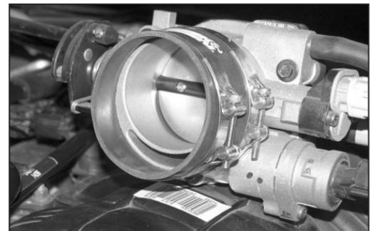
21. Install the silicone hose (084031) onto the throttle body and secure with the provided hose clamp.
