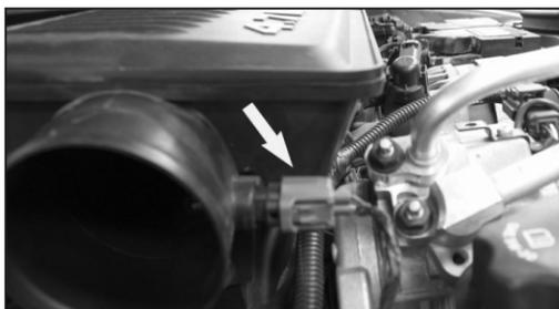
20a. Disconnect the air temperature electrical connection.
