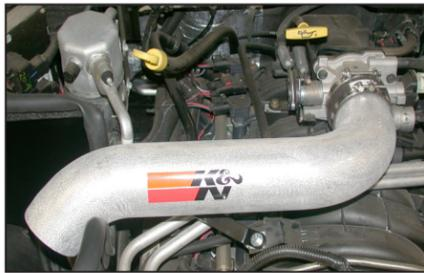
21. Install the K&N intake tube into the silicone hose at the throttle body and position so that the mounting bracket aligns with the plenum mounting location. Then secure with the provided hardware.
