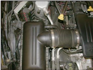
2. Loosen the hose clamp at the throttle body and the airbox mounting nut and then disconnect the crankcase vent hose from the inline fitting.
