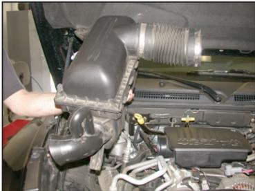
3. Disconnect the stock intake tube from the intake plenum and lift to remove the airbox assembly from the vehicle as shown.
