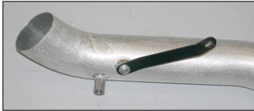
20. Install the tube mounting bracket (010121) onto the K&N intake tube as shown using the provided hardware.
