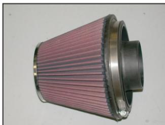
24. Install the air filter adapter into the K&N air filter as shown and secure with the provided hose clamp.
