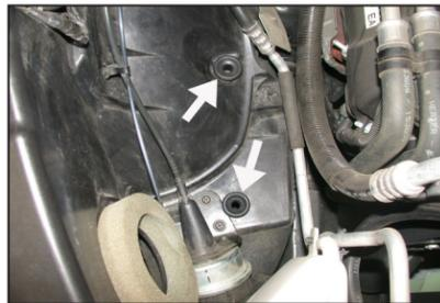
7. Pull the two airbox mounting grommets shown from the inner fender.
