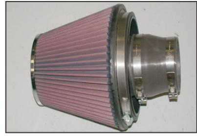
25. Install the silicone hose (084055) onto air filter adapter as shown and secure with the provided hose clamp as shown.
