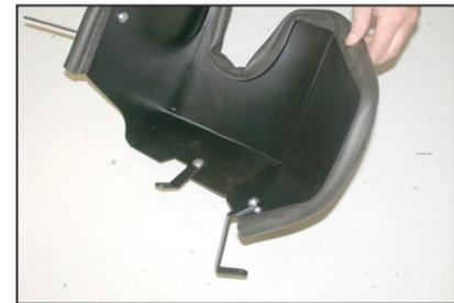
11. Install the "C" bracket (010123) onto the heat shield with the provided hardware as shown.
