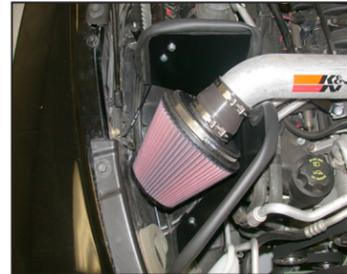
26. Install the air filter assembly onto the K&N intake tube and secure with the provided hose clamp as shown.
