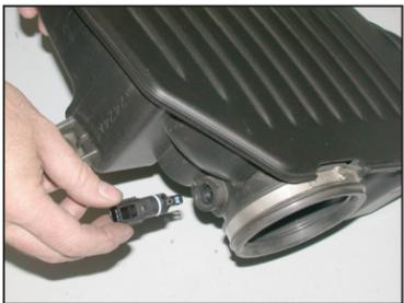
16. Twist the air temperature sensor counter clockwise and remove it from the stock intake plenum.
