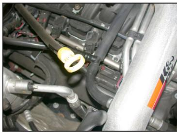
23. Install the provided crankcase vent hose onto the factory crankcase vent fitting and then onto the K&N intake tube as shown.
