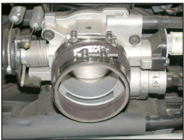
15. Install the provided silicone hose (084031) onto the throttle body and secure with the provided hose clamp as shown.
