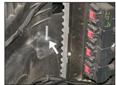
12. Install the provided 5/16" washer onto the airbox mounting stud as shown.
