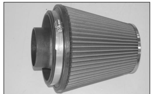
26. Install the filter adapter into the air filter as shown, secure with the provided hose clamp.
