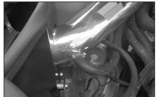
25. Connect the crankcase vent hose onto the K&N® intake tube as shown and secure with the provided hose clamp.
