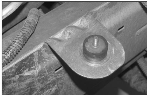
19. Using the two fender washers and one rubber washer, install the 6mm male/female rubber mounted stud onto the lower airbox mount as shown.
