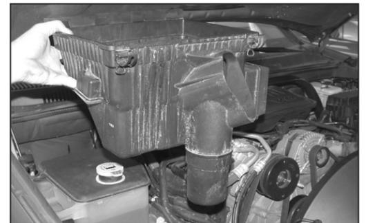
9. Remove the lower airbox from the vehicle as shown.
