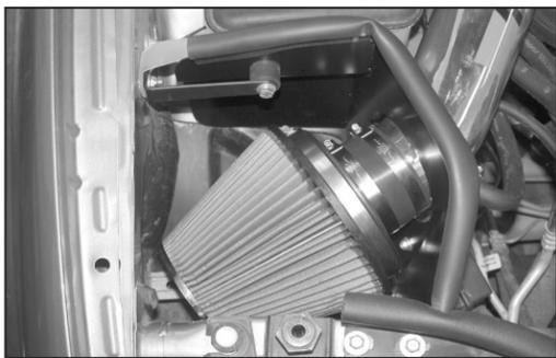
28. Install the air filter assembly onto the K&N® intake tube as shown and secure with the provided hose clamp.
