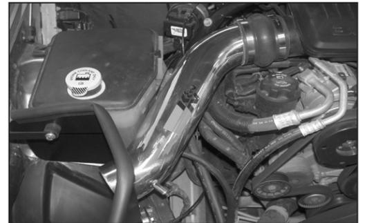
24. Install the K&N® intake tube into the silicone hose at the throttle body and onto the bracket. Secure the tube with the provided hose clamp and hardware.
