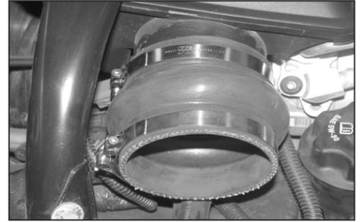
23. Install the silicone hose (084056) onto the intake plenum and secure with the provided hose clamp as shown.
