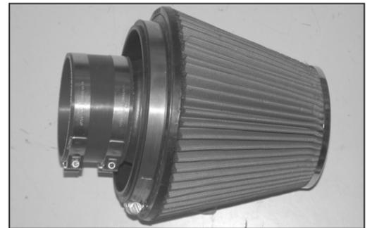
27. Install the silicone hose (08698) onto the air filter assembly and secure with the provided hose clamp.
