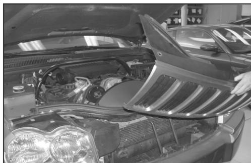
6. Remove the six grill retaining clips from the grill, then tilt the grill forward and remove from the vehicle.
