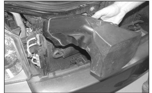
7. Pull the fresh air duct to disconnect it from the airbox and then remove it from the vehicle.
