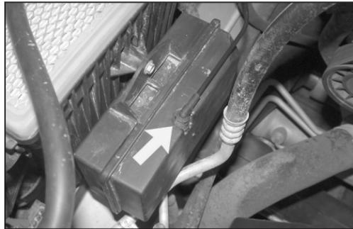
4. On vehicles equipped disconnect the vacuum canister hose shown.
