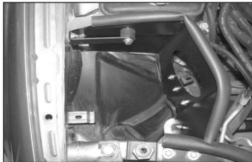
21. Install the heat shield assembly into the vehicle and secure it to the mounting locations with the provided hardware.
