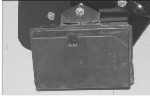
17. On vehicles equipped with vacuum reservoir, using the provided spacer, install the vacuum reservoir onto the heat shield as shown.
