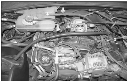
33. Install the K&N® crank case vent hose assembly onto the two check valves as shown.
