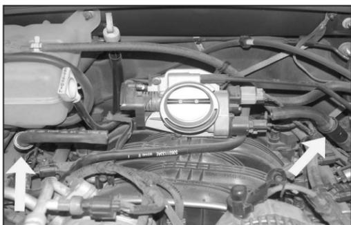
31. On vehicles equipped with an intake resonator, remove the two crank case vent hoses from the two check valves shown.
