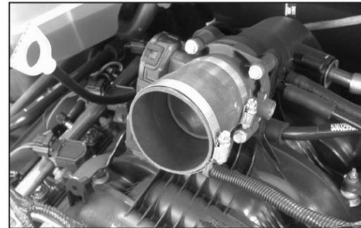
23a. On 2007 and later vehicles with a plastic throttle body, install the silicone hose (08096) onto the throttle body and secure with the provided hose clamp.
