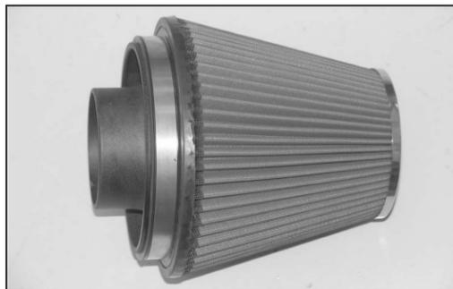
37. Install the filter adapter into the air filter as shown and secure with provided hose clamp.
