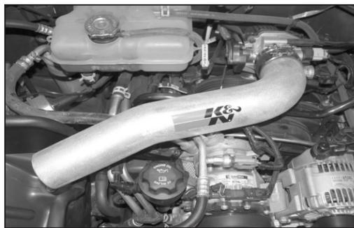
34. Reinstall the K&N® intake tube and secure with the provided hardware.
