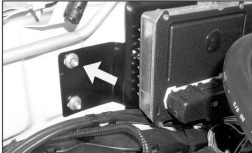
11. Remove nut from inner fender on vehicles that come equipped with a TCM.
