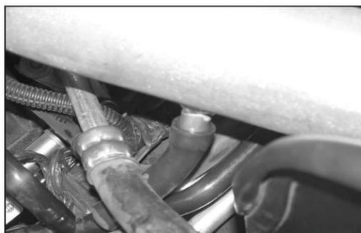
36. Connect the supplied crank case vent hose onto the K&N® intake tube.
