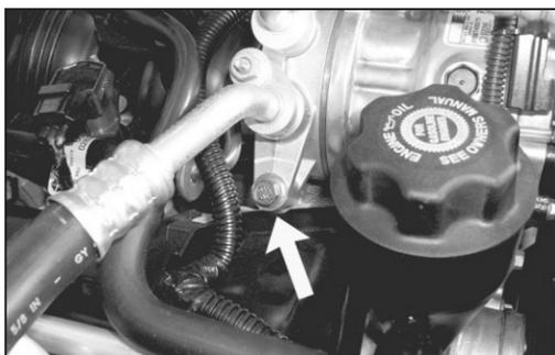
21. Remove the A/C compressor-mounting bolt.
