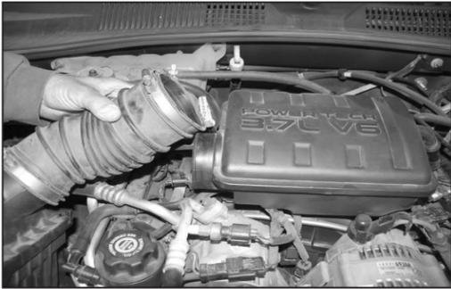
2. On vehicles with an intake resonator, loosen the hose clamp at the resonator and remove the intake hose as shown.
