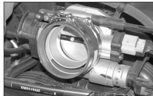
23. Install the silicone hose (084031) onto the throttle body with supplied hose clamps.
