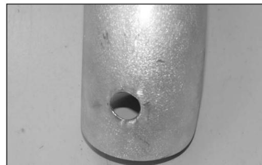
26. Drill a 3/4" id hole at the marked location on the intake tube.
