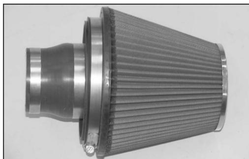
38. Install the silicone (084055) onto the filter adapter and secure with the provided hose clamp.
