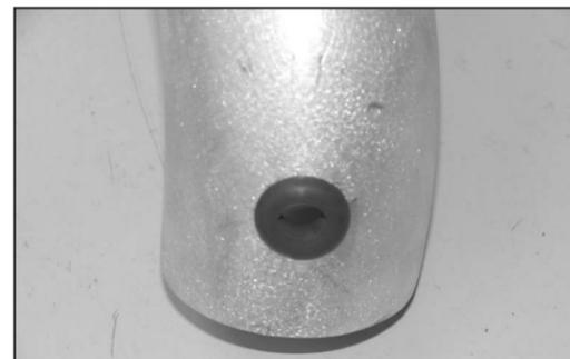
27. Install the supplied rubber grommet into the hole drilled into the K&N® intake tube as shown.
