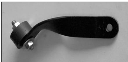
15. Assemble the bracket and rubber mounted stud as shown.
