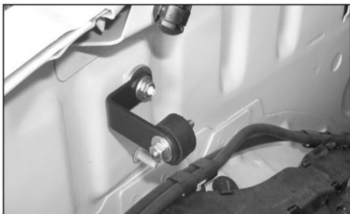
13. On vehicles that did not come with a TCM, mount "L" bracket onto existing stud with the provided hardware.
