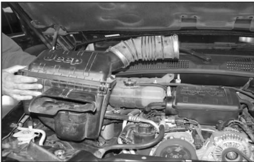
3. Firmly lift up to disengage the air box from the mounting grommets and remove the air box from the vehicle.
