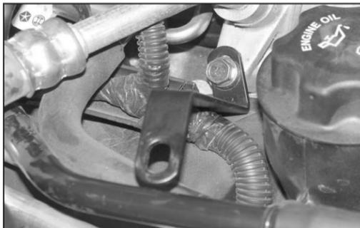
22. Using the bolt removed in step #21, install the tube mounting bracket (010064) onto the A/C pump as shown.
