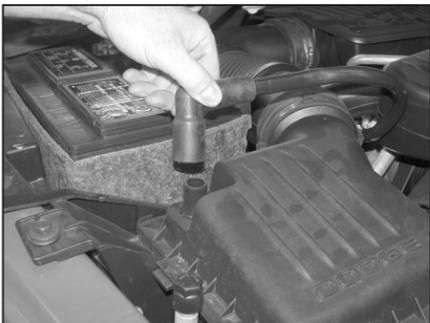
2a. On 2006 and later vehicles, disconnect the crankcase vent tube from the rear of the intake manifold.
