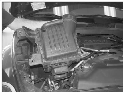
5. Pull up firmly to dislodge the airbox from mounting grommet, and remove the airbox from the vehicle.
