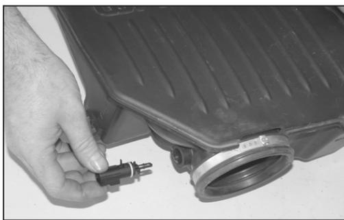
15. Twist the temp sensor counter clockwise to unlock and remove the temp sensor from the factory resonator.
