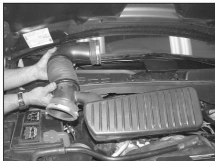
3. Loosen the intake tube hose clamps and remove the intake tube assembly from the vehicle.
