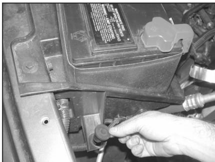
12. Install the 3/8" threaded insert provided into the airbox mounting grommet hole vacated in step #11.
