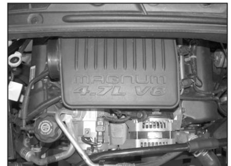
7. Remove the two 10mm resonator retaining bolts, then remove the resonator from the vehicle.
