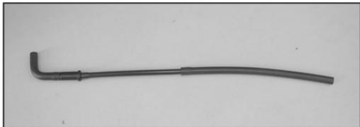
7c. Install the provided silicone hose onto the cut crankcase vent hose as shown and then reconnect the hose assembly onto the intake manifold.
