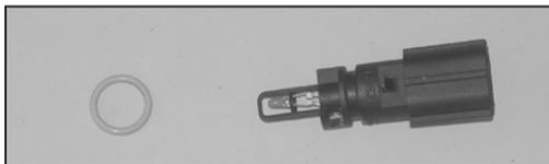
16. Remove the O-ring from the air temp sensor as shown.
