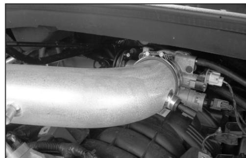
19. Slide the K&N® intake tube into the silicone hose on the throttle body as shown.
