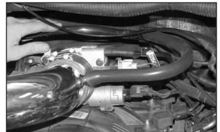
38. Connect the provided vent hose onto the "T" fitting, then connect the other end onto the intake tube.
