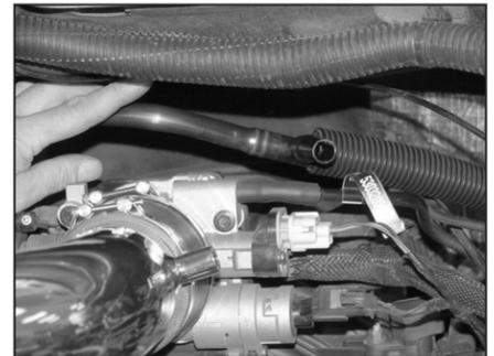
37. Reinstall the vent tube assembly into the rubber fittings in each valve cover so that the "T" fitting is now on the drivers side of the engine facing forward.
