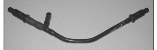
36. Rotate the long side of the vent tube assembly 180° as shown.
