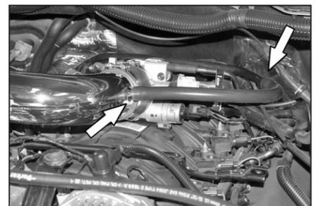
40. On models with the crank case vent tube connected to the passenger side valve cover, connect the provided silicone hose to the factory vent tube. Then, route the crank case vent tube assembly behind the throttle body as shown. Connect the open end onto the K&N® intake tube.
