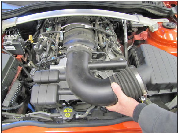
6. Remove the stock intake tube as shown.
