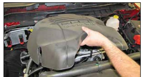
6. Lift up the engine cover and remove it from the vehicle.
