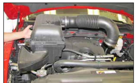
5. Disconnect the factory intake tube from the throttle body, then lift up the intake assembly and remove it from the vehicle.
