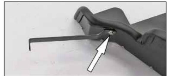
18. Install the heat shield mounting bracket (083103-1) onto the heat shield using the provided hardware.
