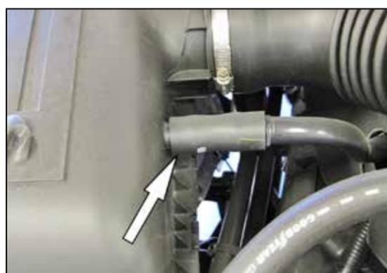
4. Disconnect the crank case vent hose from the upper air filter housing.
