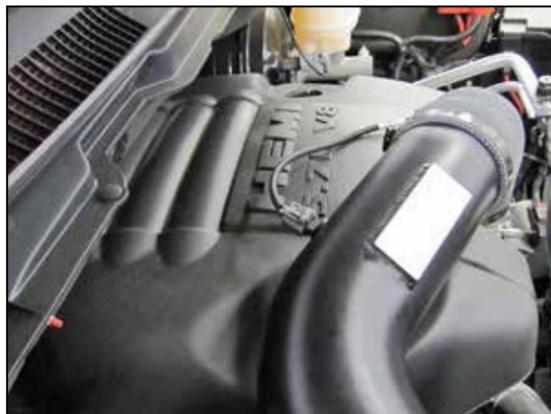
29. Choose the appropriate inlet air temperature sensor extension harness and then connect. Install it to the inlet air temperature sensor and vehicle harness.
