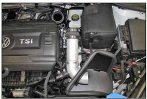
17. Install the intake tube assembly into the heat shield and secure it to the bracket installed onto the heat shield using the provided hardware.
