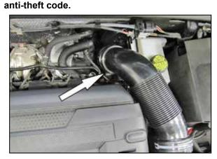
2. Loosen the hose clamp that secures the intake tube to the turbo inlet.
