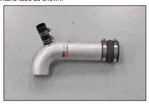
16. Install the remaining coupling hose (08185) onto the K&N<sup>®</sup> intake tube as shown.
