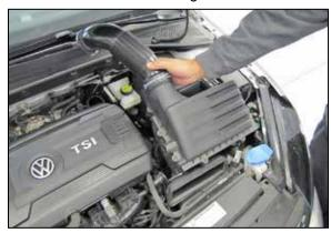
4. Lift up the air filter housing to dislodge it from the mounting grommets and then rotate the assembly up from the rear to disengage it from the fresh air intake and remove it from the vehicle.
