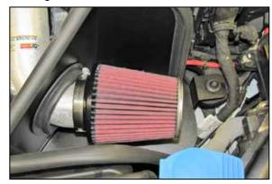
20. Install the K&N® air filter onto the intake tube and secure with the provided hose clamp.
