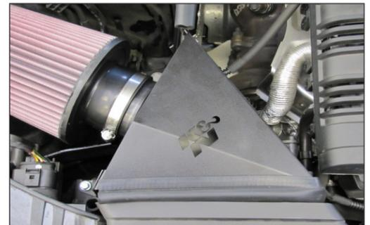
23. Using the provided hardware, secure the fresh air scoop to the heat shield as shown.
