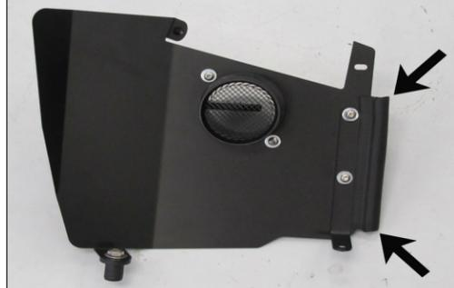
14. Install the 7" section of edge trim onto the heat shield as shown.
