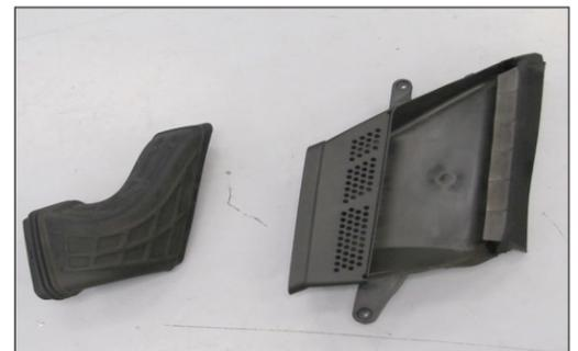
24. Separate the fresh air bellows from the fresh air scoop as shown.
