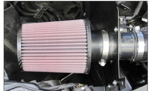
21. Install the K&N® air filter onto mass air sensor and secure with the provided hose clamp.
