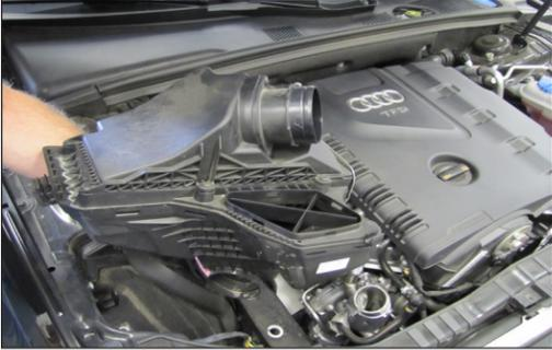
8. Pull up the air box and remove it from the vehicle.
