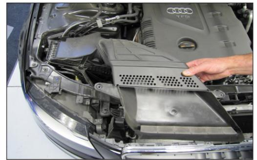
5. Unsnap the fresh air scoop from the air box and then remove the scoop from the vehicle.
