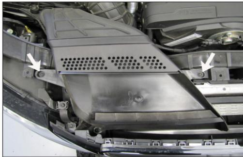
4. Remove the two screws which secure the fresh air scoop to the core support.
