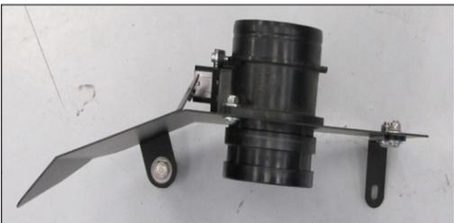
12. Install the mass air sensor into the heat shield as shown and secure with the provided hardware.
