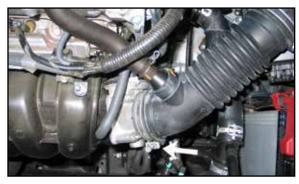
5. Loosen the hose clamp which secures the intake tube to the throttle body.
