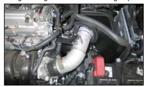
17. Install the K&N® intake tube into the silicone hose at the throttle body and align with the bracket installed in the previous step. Secure the intake tube with the provided hose clamp and hardware.
