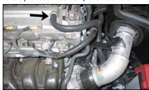
18. Install the crank case vent hose onto the valve cover port and then onto the K&N® intake tube.
