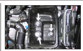
7. Remove the three lower air box retaining bolts. Then unclip the wiring harness from the rear of the air box and remove the lower air box housing from the vehicle.
