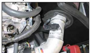
19. Route the mass air electrical harness through the heat shield as shown and then reconnect the mass air sensor electrical connection.
