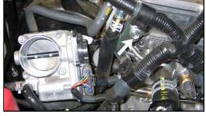
8. Remove the bolt shown which secures the engine wiring harness to the engine.
