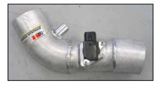
15. Install the mass air sensor into the K&N<sup>®</sup> intake tube and secure with the provided hardware.
