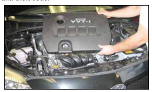
2. Pull up firmly to dislodge the engine cover from the mounting grommets and then remove the cover from the engine.
