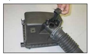
14. Remove the two screws that secure the mass air sensor to the upper air box and then remove the mass air sensor as shown.
