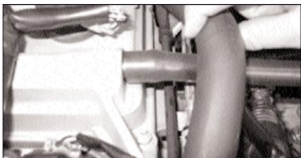
20. Fit the provided silicone breather hose to the breather tube on the valve cover.
