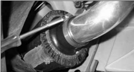
24. From underneath the car, slide the filter onto the intake tube & tighten the hose clamp.
