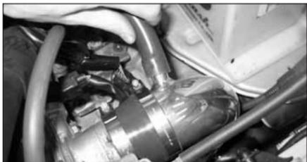
21. Fit the other end of the breather hose onto the intake tube.
