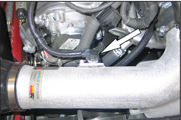
29. Reconnect the mass air sensor electrical connection.
