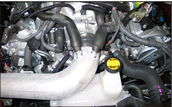
28. Connect the crank case vent hoses to the K&N® intake tube and secure with the factory spring clamps.
