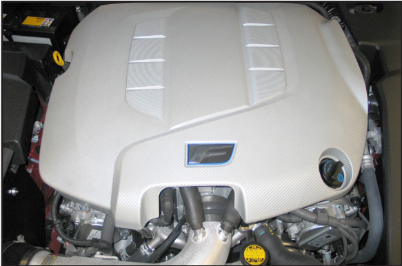
36. Reinstall the engine cover.
