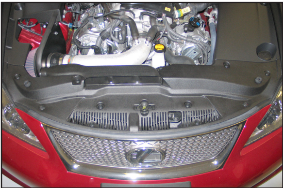
35. Install the front cover and secure with the factory retaining clips.
