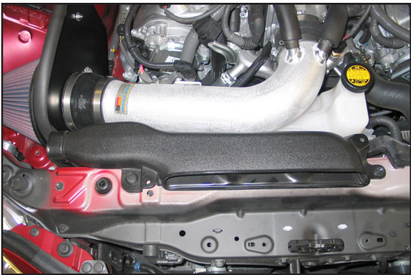
33. Install the fresh air intake scoop using the factory bolt and retaining clip.
