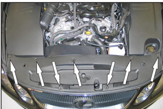
3. Depress the center locking button to release seven core support fasteners.
