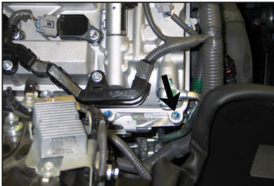
28. Remove the valve cover mounting bolt shown.
