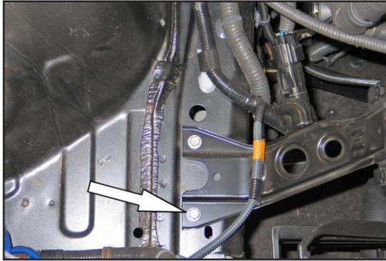
17. Remove the relay bracket mounting bolt shown.
