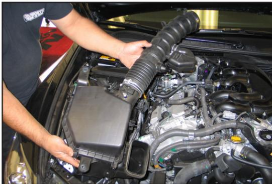
12. Remove the complete intake assembly.
