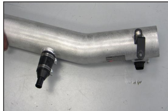
26. Install the "Z" (070992) onto the K&N® intake tube as shown.
