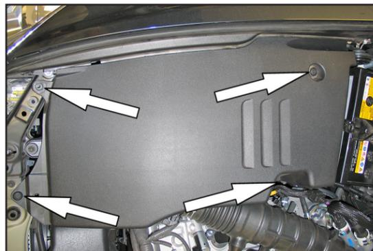
5. Depress the center locking button on the two air filter cover fasteners, remove the two fasteners and unscrew plastic screw shown. Then remove the cover from the vehicle.
