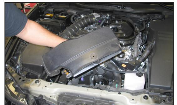
7. Remove the fresh air supply from the core support as shown.
