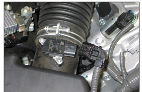
8. Disconnect the mass air sensor electrical connection and unhook the wiring harness from the air box.
