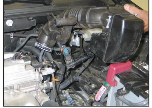
9. Release the spring clamp that secures the stock intake tube at the throttle body. Then, remove the complete intake tube assembly as shown.
