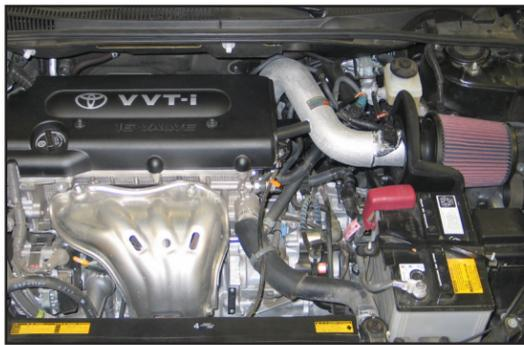
28. Reconnect the vehicle's negative battery cable. Check to ensure all hose clamps and fittings are properly tightened and positioned correctly before starting the vehicle.
