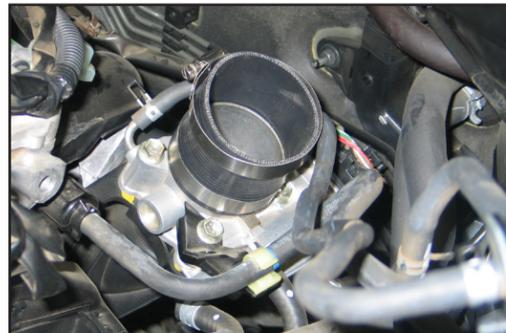
18. Install silicone hose (#084016) onto the throttle body and secure with the provided hose clamp.
