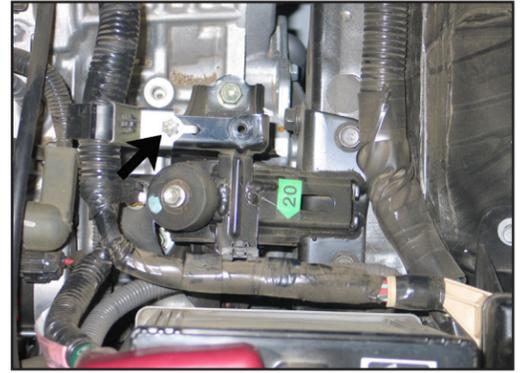
10. Remove the bolt that secures the wiring harness as shown.
