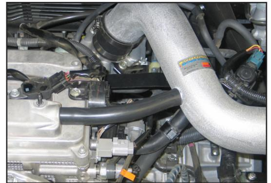
24. Install the provided crank case vent hose as shown.
