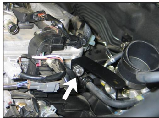
19. Install intake tube mounting bracket (#26661) onto the cylinder head and secure with the provided hardware as shown.
