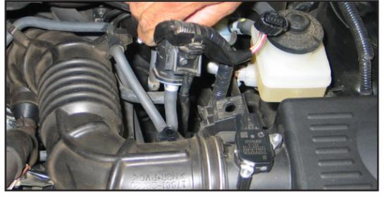
4. Un-hook the EVAP solenoid valve from the stock intake tube as shown.
