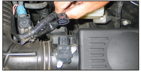
3. Depress the locking tab on the mass air sensor electrical connection, then disconnect the mass air sensor electrical connector.
