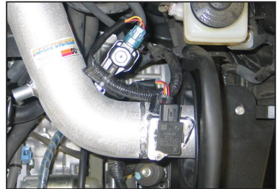
23. Secure the EVAP mounting bracket to the intake tube with the provided hardware.
