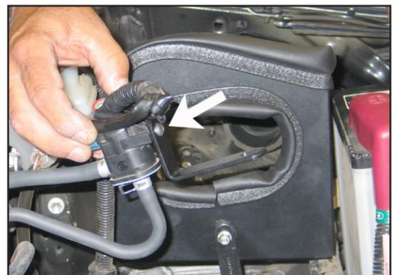
21. Secure the provided bracket (#070622) to the EVAP solenoid valve as shown.
