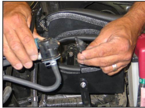
20. Remove the screw that secures the mounting bracket to the EVAP valve, then remove the mounting bracket as shown.
