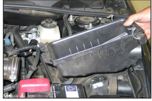
7. Remove the three lower air box mounting bolts shown, then remove the lower air box from the vehicle.
