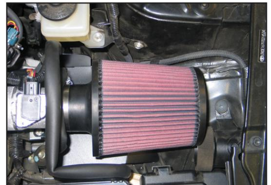
25. Install the K&N® air filter onto the K&N® intake tube and secure with the provided hose clamp.
