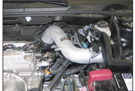
22. Install the K&N® intake tube into the silicone hose at the throttle body and align with the mounting bracket. Secure the intake tube with the provided hardware and hose clamp as shown.
