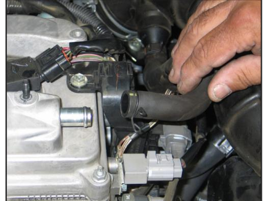
8. Un-hook the crank case vent hose from the valve cover as shown.
