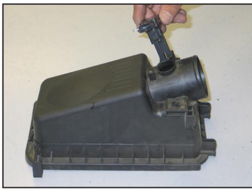
16. Remove the screws that secure the mass air sensor to the upper air box, then remove the mass air sensor as shown.
