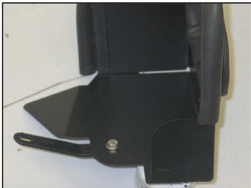
13. Install heat shield mounting bracket (#26662) onto the heat shield using the provided hardware as shown.
