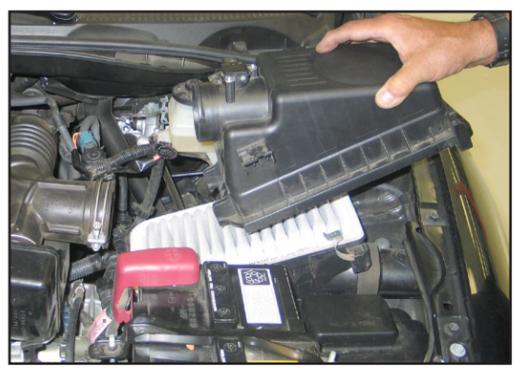
6. Un-hook the upper air box mounting clips, then remove the upper air box as shown.
