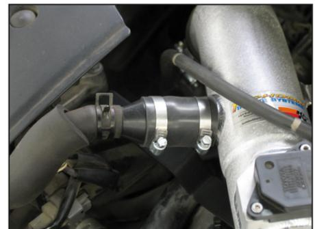
22. Install the crank case vent hose/chamber into the silicone hose installed onto the K&N intake tube in step 19; secure with the provided hose clamp.
