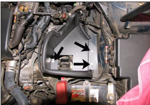
12. Set the heat shield into position on the lower air box mount and inner fender. Using the provided hardware, secure the heat shield to the three original lower air box mount's threaded holes.
