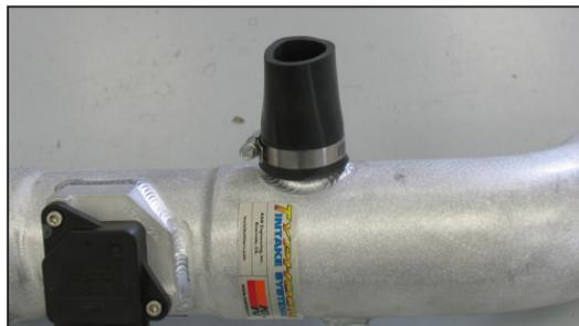
17. Install the provided silicone hose (084074) onto the K&N intake tube and secure with the provided hose clamp.
