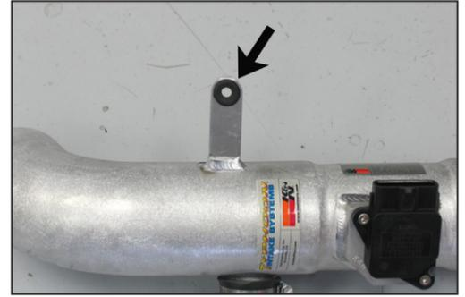
20. Install the provided grommet into the welded bracket on the K&N intake tube.
