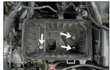
7. Remove the three lower air box mounting bolts; then, release the two wiring harness mounting clips which secure the wiring harness to the lower air box.
