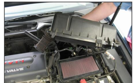
6. Release the clamp that secures the stock intake tube to the throttle body. Then, remove the factory intake tube/upper air box as shown in the photograph.
