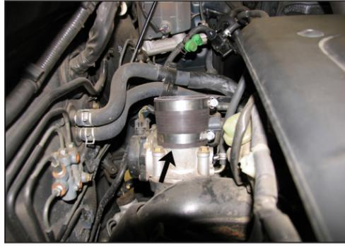
14. Install the supplied silicone hose (084016) onto the throttle body and secure with the supplied hose clamp.
