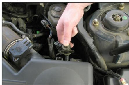
5. Loosen the two upper air box mounting bolts, then remove the screw that secures the "EVAP canister closed valve" to the upper airbox as shown in the photograph.
