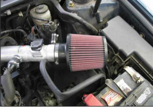
25. Install the K&N® air filter onto the intake tube; secure with the provided hose clamp.
