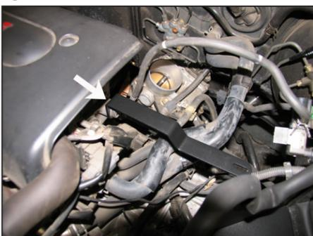
13. Install the intake tube mounting bracket (26651) onto the engine using the provided hardware as shown in the photograph.
