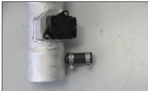
19. Install the newly cut 1-3/4" long silicone hose (08415) onto the K&N intake tube and secure with the provided hose clamp as shown in the photograph.
