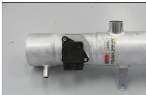
16. Install the mass air sensor into the K&N intake tube and secure with provided hardware.
