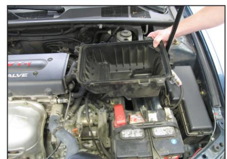
8. Remove the lower air box from its place of attachment as shown in the photograph.
