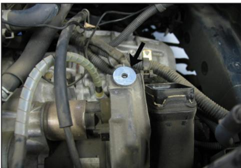
11. Place the provided rubber washer and fender washer onto the lower air box mount as shown in the photograph.
