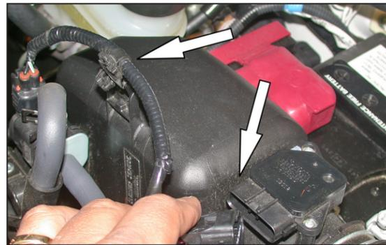
2. Disconnect the mass air sensor electrical connection and unclip the wire harness from the side of the air cleaner assembly as shown. **NOTE: On '06 & later models, unclip the MAS wiring harness from air box lid.**
