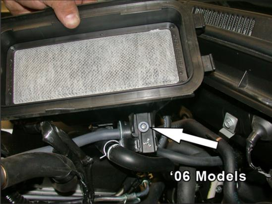
6. Release the clamps on the upper air cleaner assembly, then, remove the upper air cleaner assembly as shown.
