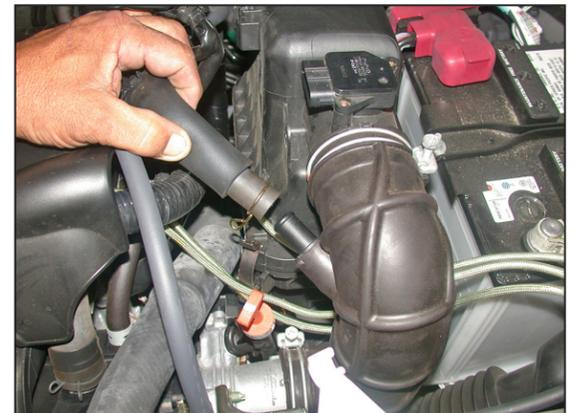
4. Disconnect the crank case vent hose from the stock intake tube as shown.
