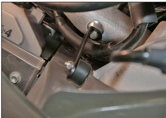
25. Line up the bracket from step 20 with the threaded boss on the K&N® Typhoon® cold air tube, then secure it using the provided hardware as shown, but do not tighten at this time.
