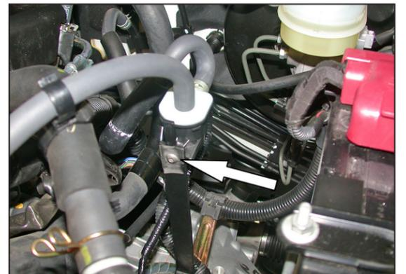
18. Slide the PWM vacuum switching valve onto the "L" bracket from the previous step.
