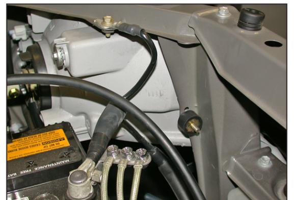
19. Install the provided rubber mounted stud into threaded hole on the radiator core support from step 8.
