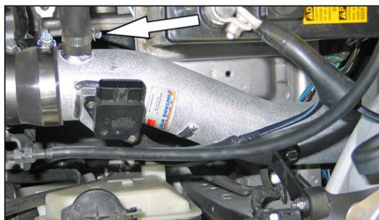
28. Slide the hose mender into the stock crank case vent hose, then, connect the other end to the vent on the K&N® Typhoon® cold air tube as shown.
