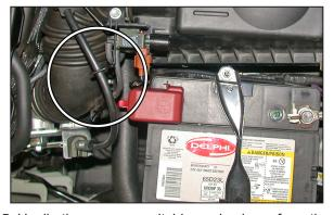
5. Unclip the vacuum switching valve hose from the intake tube.
