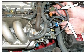
23. On 2003 model year vehicles, remove the vacuum hose from the intake manifold as shown. On '04-06 models, remove vacuum hose from the vacuum switching valve and the "T" fitting as shown.
