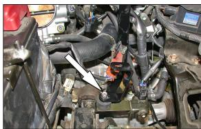
31. Install the "C" bracket to the rubber mounted stud using the provided hardware, but do not tighten completely.
