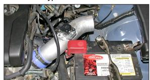
33. Slide the tube onto the throttle body but do not tighten completely at this time.
