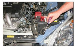
18. Remove the push clip that secures the air inlet duct to the radiator core support as shown.
