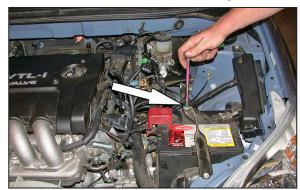
16. Loosen the battery hold down bracket as shown.
