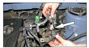
26. Remove the stock hose from the EVAP OBD canister closed valve as shown.
