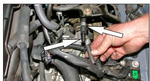
27. Insert the provided hose mender into the stock hose from step 25, then, slide the provided silicone hose onto the end of the hose mender as shown.
