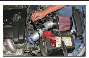
40. Reconnect the mass air sensor electrical connection as shown.
