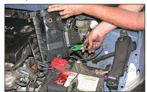
14. Tilt the lower air cleaner assembly upwards to unclip the wire harness as shown.
