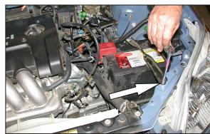
21. Reinstall the battery hold down bracket as shown.
