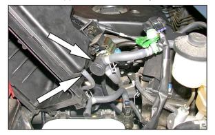
10. Unclip the upper air cleaner assembly, then, tilt upwards to unclip the PWM vacuum switching valve and the vacuum hose as shown.
