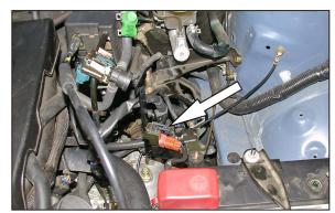
30. Secure the vacuum switching valve to the "L" bracket using the screw removed in step 4.
