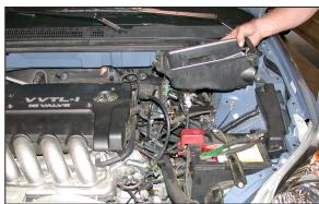
15. Remove the lower air cleaner assembly as shown.
