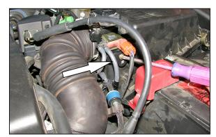
3. Remove the two screws that secure the vacuum switching valve to the air cleaner assembly as
