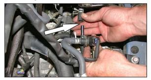
25. On vehicles equipped with the EVAP OBD canister closed valve from step #12, pull the hose clamp back and disconnect the EVAP OBD canister closed valve as shown. All others skip to setp #29.
