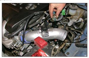
37a. On vehicles that use a clip type PWM vacuum switching valve, slide the valve onto the "L" bracket as shown.
