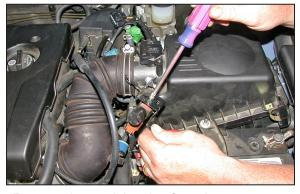
4. Remove the stock bracket from the vacuum switching valve as shown.
