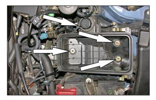
13. Loosen and remove the three bolts that secure the lower air cleaner assembly as shown. Also disconnect the vacuum hose from the butterfly valve as pictured.
