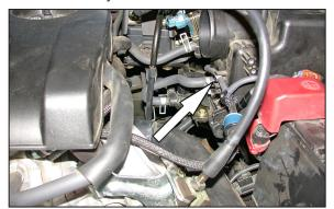
9. Unclip vacuum switching valve hoses from air box, then unclip the PWM switching valve wire harness from upper air box assembly.
