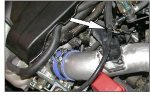
36. Slide the throttle cable into the wire hanger as shown.
