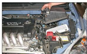
11. Remove the upper air cleaner assembly as shown.
