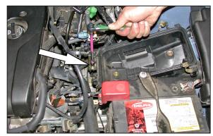
12. On vehicles equipped with EVAP canister closed valve, remove the bolt that secures the EVAP OBD canister closed valve to the lower air box assembly.
