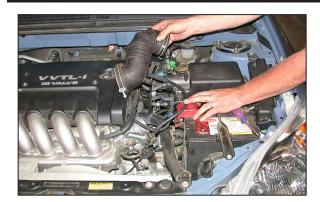
7. Loosen the hose clamps at the throttle body and at the air cleaner assembly, then, remove the stock intake tube as shown.
