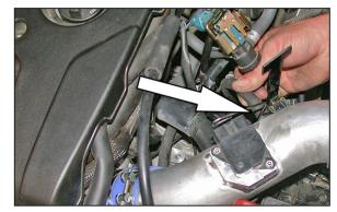
35. Slide the wire hanger onto the vent on the Typhoon® intake tube, then, on 03-04 models connect the hose from the EVAP OBD canister closed valve onto the vent as shown.
