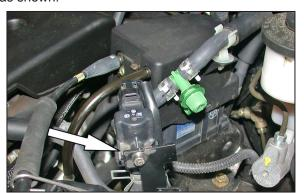
37b. On vehicles that use a screw to secure the PWM switching valve, scure the valve to the "L" bracket using the screw removed in step #6.
