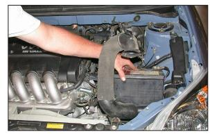
20. Tilt that battery backwards, then, remove the air inlet duct as shown.
