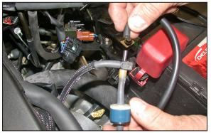
24. On 2003 model year vehicles, install the rubber cap plug onto the vent on the manifold as shown. On '04-06 models, install the rubber cap plug onto the "T" fitting as shown.
