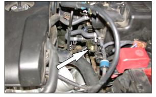
8. On vehicles equipped with an EVAP canister closed valve, disconnet the vent line from the air cleaner assembly.
