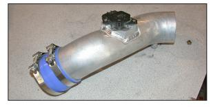
32. Install the mass air sensor into the adapter on the Typhoon® intake tube and secure with the provided hardware. Then install the silicone hose and hose clamps.
