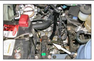
29. Secure the provided "L" bracket and the stock EVAP OBD canister closed valve bracket to the original air claner mount, using the provided rubber mounted stud.
