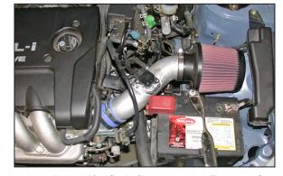
38. Install the K&N® air filter onto the Typhoon® intake tube and secure with the provided hose clamp as shown.
