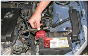
17. Remove the bolt that secures the battery hold down bracket to the radiator core support, then, remove the battery hold down bracket as shown.
