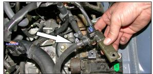
28. Slide the EVAP OBD canister closed valve into the hose from step 27.
