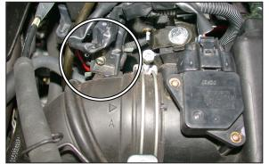
6. Remove screw from PWM switching valve.
