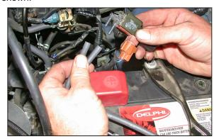
22. Disconnect the two vacuum hoses from the vacuum switching valve as shown.
