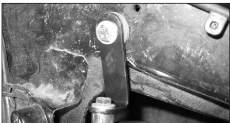
19. Mount the angled bracket onto the lower threaded hole in the inner fender using the washer, rubber washer and M6 bolt supplied. Do not fully tighten at this moment.
