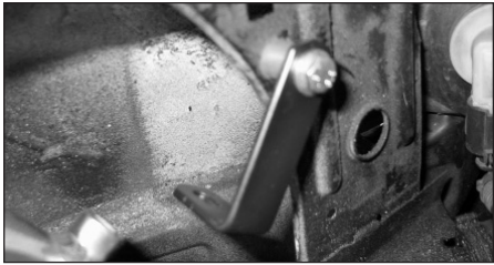
20. Mount the L bracket onto the inner fender using the M6 bolt, washer, spacer, large washer and M6 nutt supplied. Do not fully tighten at this moment.
