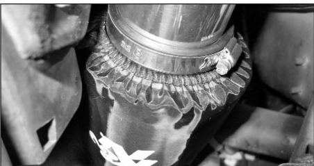
24. Mount the filter onto the B tube using the hose clamp supplied.
