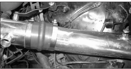
25. Align the A and the B tubes for maximum clearance, now tighten all hose clamps, bolts and nuts.
