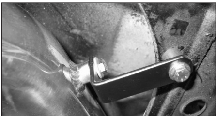
21. Mount the tube onto the L bracket using the hardware supplied. Do not fully tighten at this moment.
