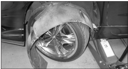
22. Taking the necessary safty precautions raise the front of the vehicle and remove the wheel arch liner as shown .
