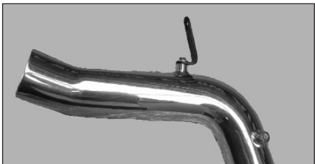
17. Mount the angled bracket onto the B tube using the hardware supplied. Do not fully tighten at this moment.
