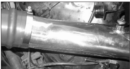
18. Feed the B tube into the inner fender and mount the B tube into the sleeve using a #44 hoseclamp supplied. Do not fully tighten at this moment.
