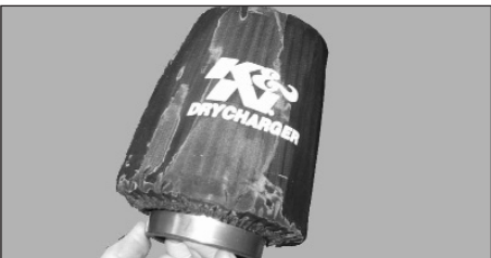
23. Fit the drycharger over the filter as shown. NOTE: The Drycharger's water repellent properties will last up to two years. See the parts list to re-order Drycharger if necessary.
