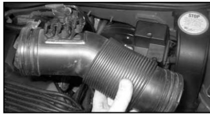
7. Depress the throttle body hose clamp and remove the complete intake tube from the vehicle as shown.
