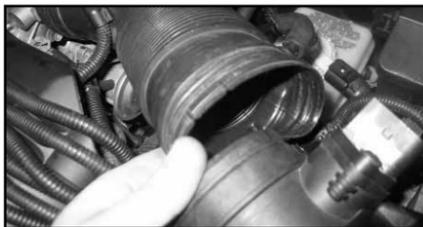
3. Depress the hose clamp to remove the intake tube from the MAS.
