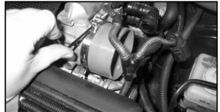
15. Install the silicone hose onto the throttle body using the #48 hose clamp supplied.
