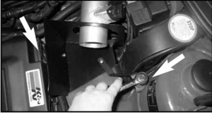
18. Mount the heat shield onto the air box support points using the hardware supplied. (do not fully tighten yet!)
