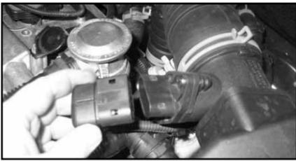
2. Disconnect the mass air sensor (MAS) electrical connection as shown.
