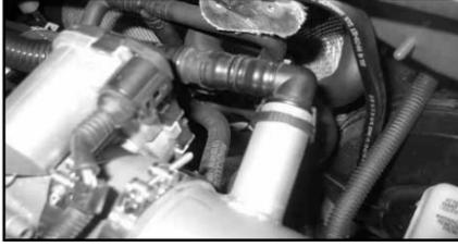
23. Reconnect the crank case vent hose to the intake tube.
