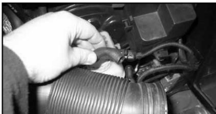
5. Remove the small breather hose from the intake tube as shown.
