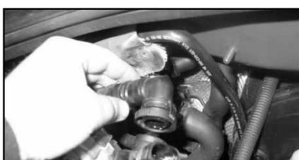
6. Disconnect the crank case vent switch and the crank case hose from the intake tube as shown.
