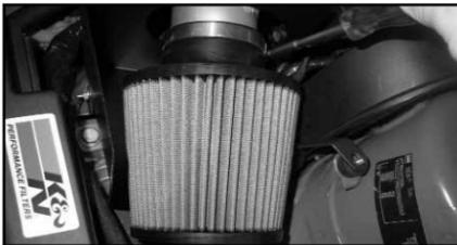
26. Fit the filter onto the intake tube using the hose clamp supplied.
