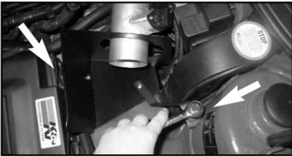
21. Mount the heat shield back on the air box support points using the hardware supplied.
