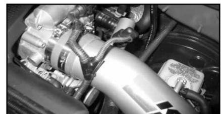
16. Fit the new intake tube into the silicone hose using the #48 hose clamp supplied. (do not fully tighten at this moment.)
