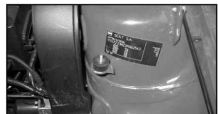
12. Mount the rubber vibration stud onto the airbox support bracket.
