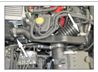
4. Loosen the rear hose clamp and release the spring clamp securing the sound to the drum and intake tube. Then remove the sound tube from the vehicle.
