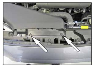
2. Remove the two clips securing the fresh air intake duct and then remove the intake duct from the vehicle.
