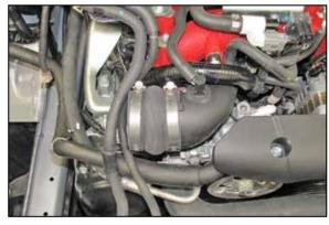
14. Install the provided coupling hose (08185) onto the turbo inlet and secure with the provided hose
