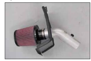
15. Install the K&N<sup>®</sup> intake tube through the heat shield as shown and then install the K&N® air filter onto the intake tube and secure with the provided hose clamp.
