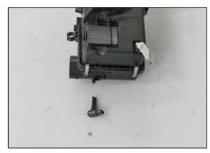
10. Remove the two screws securing the mass air sensor into the air filter housing and then remove the sensor.
