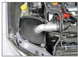
16. Install the intake assembly onto the frame and inner fender then install the intake tube into the coupling hose. Adjust the tube and heat shield for best fit and secure with the provided hose clamp and hardware.
