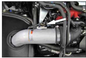
17. Reconnect the mass air sensor electrical connection.
