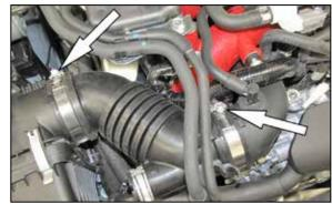
8. Loosen the two hose clamps securing the intake tube and then remove the intake tube from the vehicle.
