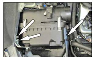
9. Remove the air box mounting bolt and nuts shown and then remove the complete air filter assembly.
