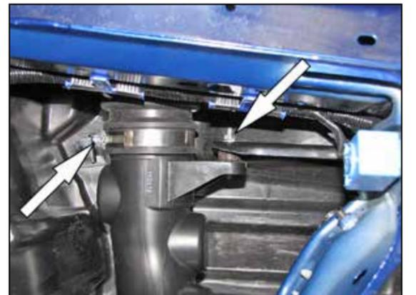
6. Loosen the hose clamp securing the intake tube and remove the nut on the lower mount.
