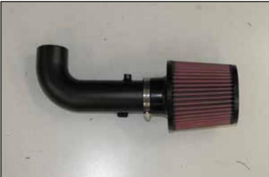
10. Install the K&N® air filter onto the K&N® intake tube and secure it with the provided hose clamp.
