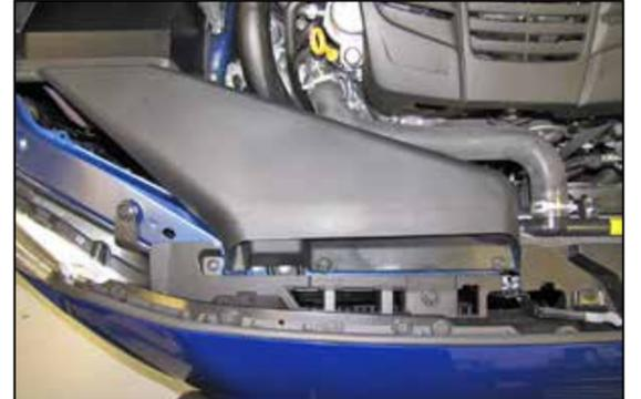
18. Install the fresh air intake scoop and secure with the factory retaining clips.
