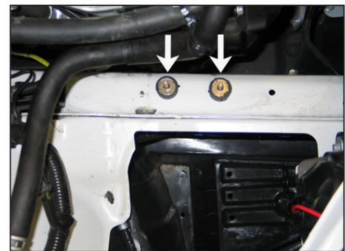
7. Install the two rubber mounted studs into the inner fender as shown.
