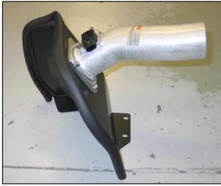
14. Install the K&N® intake tube onto the studs and secure with the provided nuts and washers.
