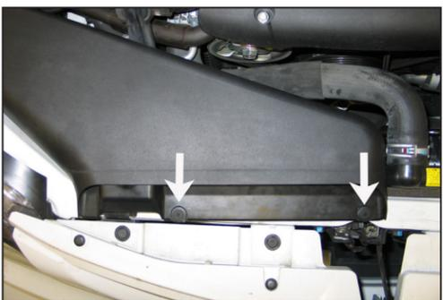
2. Remove the two fasteners which retain the fresh air inlet scoop and then remove the fresh air inlet scoop from the vehicle as shown.
