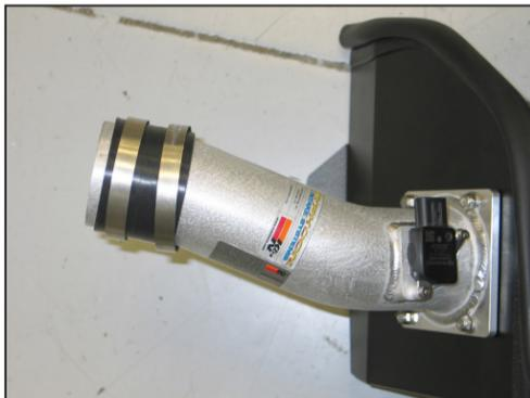
16. Install the provided silicone hose (08440) onto the intake tube as shown.
