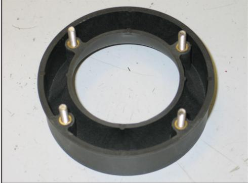
11. Install the four 6mm studs into the filter adapter as shown.
