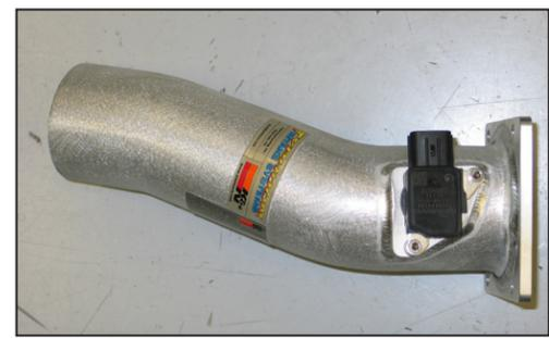
9. Install the mass air sensor into the K&N® intake tube and secure with the provided hardware.
