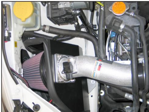
17. Install the K&N® intake kit so that the heat shield rests on the rubber mounted studs installed during step #7. Secure the heat shield with the provided hardware. Slide the silicone hose onto the turbo inlet and secure with the provided hose clamp.
