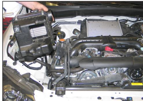
6. Remove the airbox assembly from the vehicle.
