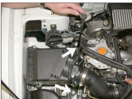
4. Loosen and remove the two bolts on the air cleaner as shown.
