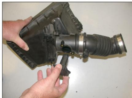
7. Remove the mass air sensor from the air cleaner as shown.
