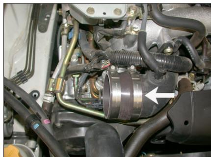
8. Install the silicone hose and hose clamps onto the turbo charger inlet tube as shown.
