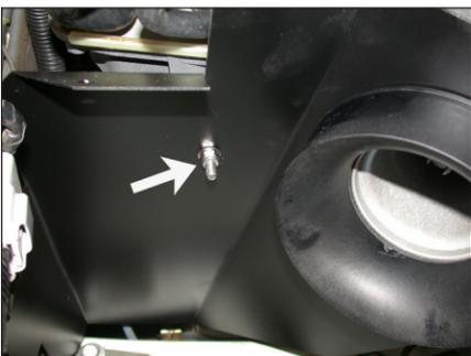
17. Secure the heat shield to the "Z" bracket using the provided hardware as shown.
