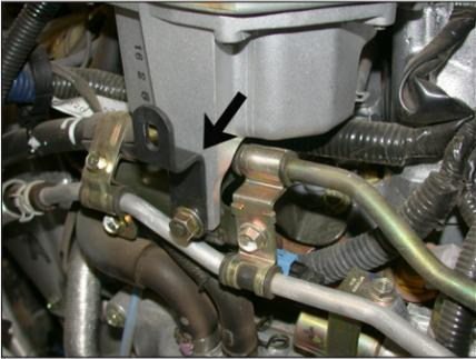
13. Install the provided "Z" bracket onto the coolant reservoir using the original nut removed in step 14.
