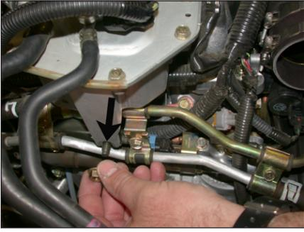
12. Remove the stock nut from the coolant reservoir as shown.
