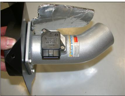
15. Install the mass air sensor into the K&N® intake tube using the provided screws as shown above.
