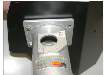
10. Assemble the tube, heat shield, filter adapter, and the remaining gasket using two of the provided hex bolts as shown above.
