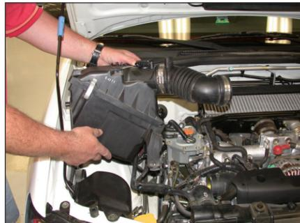
6. Remove the complete air cleaner assembly as shown.
