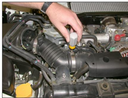
5. Loosen the hose clamp on the turbo charger inlet tube as shown.
