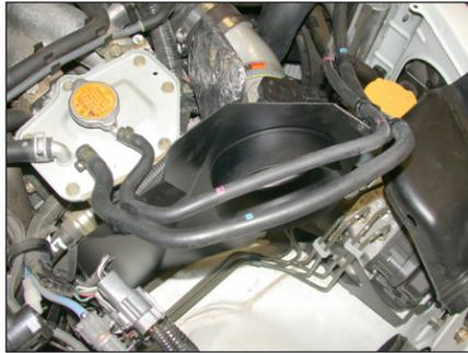
20. Install the stock coolant clips onto the two tabs on the heat shield, then clip the coolant lines onto the clips as shown.
