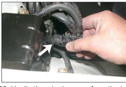
22. Unclip the wire harness from the inner fender bracket as some slack will be needed to reroute the mass air sensor electrical connection.
