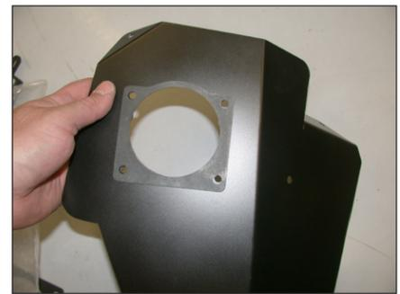
9. Install one of the provided gaskets onto the back of the heat shield as shown.
