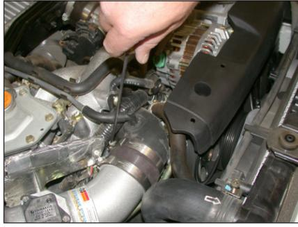
18. Tighten the hose clamp on the K&N® intake tube as shown.
