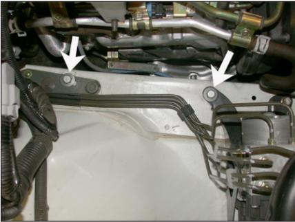
14. Reinstall the original air cleaner mounting bolts as shown above.
