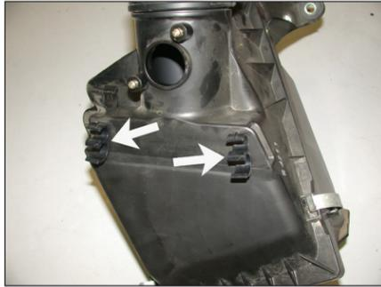
19. Remove the stock coolant clips from the stock air cleaner assembly as shown.
