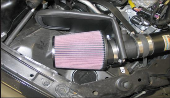
26. Install the K&N® Air Filter as shown.
