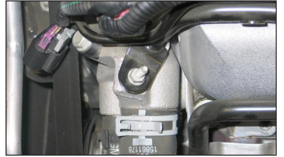
20a. On vehicles equipped with the above style heater hose tube, remove the mounting bolt shown.
