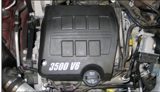
27. Install the engine cover and oil filler cap as shown.
