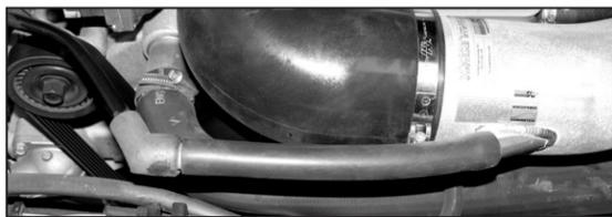
19. Install the provided vent fitting onto the supplied silicone hose as shown above, then install the crankcase vent hose onto the K&N® intake tube and the vent fitting into the stock vent line.
