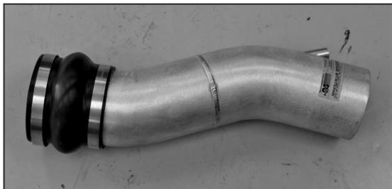
17. Install the silicone hump hose onto the intake tube as shown and secure with the provided hose clamp as shown.
