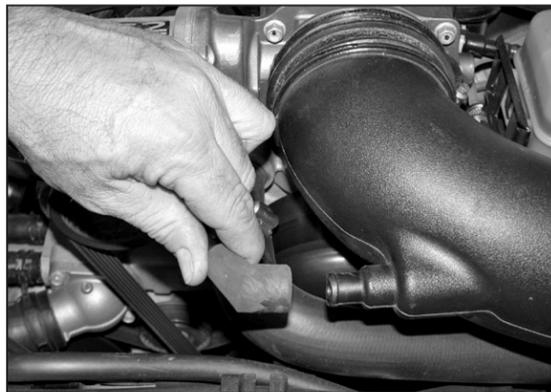
4. Disconnect the crank case vent hose from the factory intake tube as shown.
