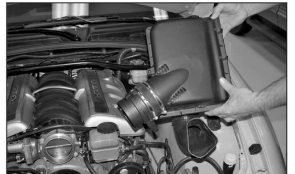
7. Pull up on the air box assembly to dislodge it from the three mounting pins and then remove the air box from the vehicle as shown.
