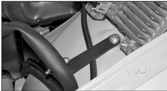
15. Install the heat shield mounting bracket onto the heat shield as shown and then secure the bracket to the inner fender at the upper air box mounting pin location as shown with the provided hardware.
