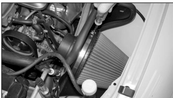
13. Install the heat shield assembly onto the inner fender and start the mount bolts in the air box mounting pin holes, then place the air filter into position. Tighten the heat shield mounting bolts and then install the air filter onto the filter adapter and secure with the provided hose clamp.
