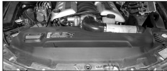
20. Reinstall the radiator cover and the five mounting clips removed in step #2.
