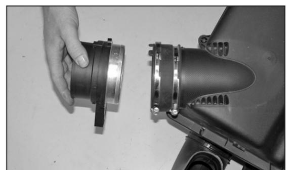
9. Loosen the hose clamp that secure the mass air sensor to the factory air box, then remove the mass air sensor from the factory air box.
