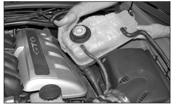
7. Pull the coolant reservoir up and away from the inner fender to release it from the retaining studs.
