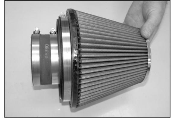
20. Install the provided silicone hose (08698) onto the filter adapter and secure with the provided hose clamp as shown.
