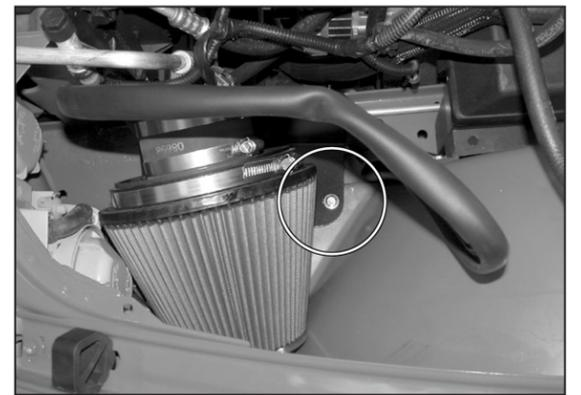
23. Secure the heat shield to the inner fender with the 6mm bolt provided.
