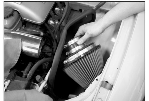
22. Set the heat shield assembly onto the inner fender, then set the filter charger assembly between the heat shield and fender as shown.
