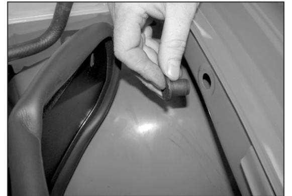
24. Install the threaded insert into inner fender as shown.
