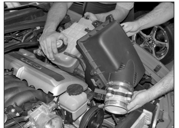
8. Have an assistant hold the coolant reservoir up, lift up on the air box assembly to release it from the retaining studs. Then remove the air box from the vehicle.
