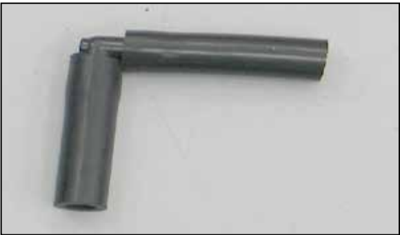
24. Connect the two 3" pieces of crank case vent hose to the 90° vent fitting as shown.
