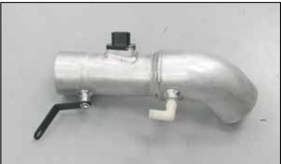
22. Install the tube mounting bracket onto the driver's side K&N® intake tube as shown and secure with the provided hardware. NOTE: The part number of the bracket will be on the leg pointing down away from the intake tube when installed properly.
