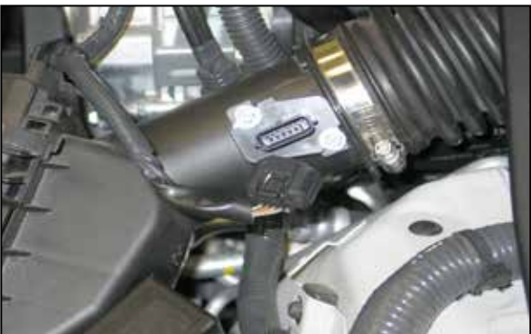
9. Disconnect the Driver's side mass air sensor and unhook the wiring harness from the air box.
