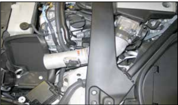
23. Install the K&N® intake tube into the silicone hose at the throttle body and align the bracket with the mounting hole in the heat shield. Adjust the tube and heat shield for proper fit and then secure with the provided hardware and hose clamp. NOTE: The tube mounting bracket is to be attached on the back side of the heat shield.
