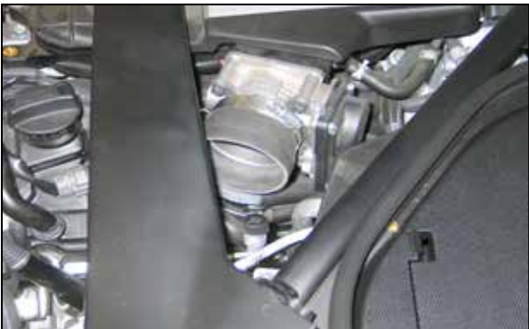
14. Install the silicone hose (084036) onto the driver's side throttle body and secure with the provided hose clamp.
