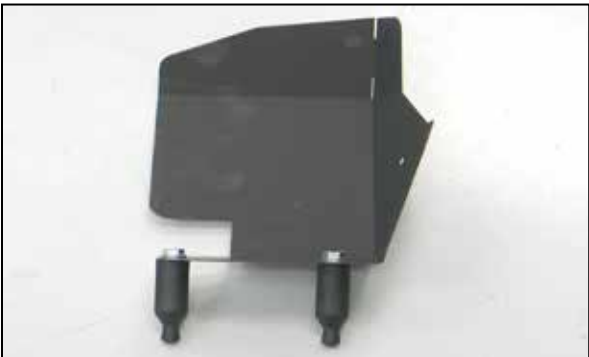
15. Install the two heat shield mounting pins onto the driver's side heat shield (074057) and secure with the provided hardware.
