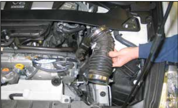
13. Remove the left side intake hose from the vehicle. NOTE: It will be necessary to release the spring clamp which secures the crank case vent hose to the valve cover port and then disconnect the crank case vent hose from the valve cover. NOTE: K&N Engineering, Inc., also recommends that customers do not discard factory air intake.
