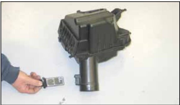
20. Remove the two screws securing the mass air sensor to the driver's side air box and then remove the mass air sensor from the air box.
