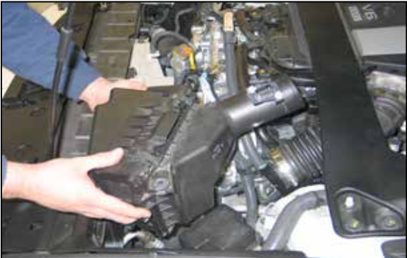
11. Remove the driver's side air box from the vehicle.
