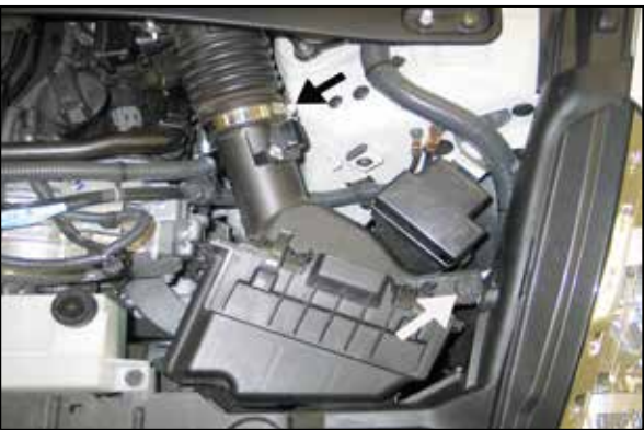
10. Loosen the hose clamp which secures the right side intake hose to the air box. Remove the bolt which secures the air box to the inner fender.
