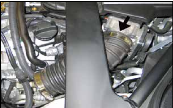
12. Loosen the hose clamp that secures the driver's side intake tube to the throttle body.
