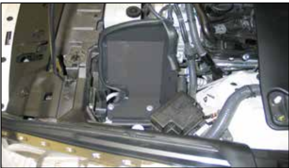
18. Install the heat shield assembly into the vehicle so that the mounting pins engage into the air box mounting grommets.
