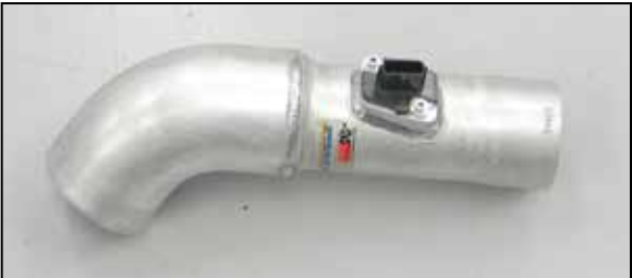
21. Install the mass air sensor into the driver's side K&N® intake tube and secure with the provided hardware.
