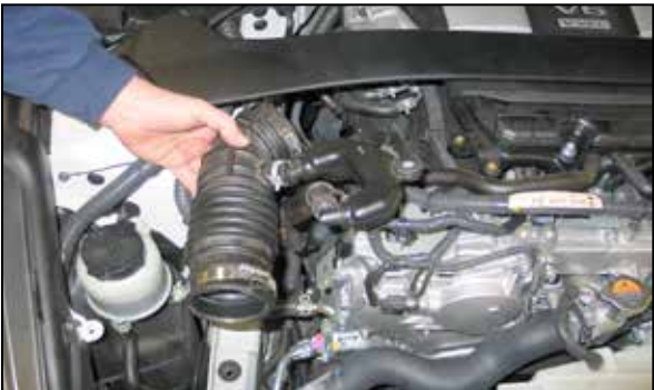
8. Remove the right side intake hose from the vehicle. NOTE: It will be necessary to release the spring clamp which secures the crank case vent hose to the valve cover port and then disconnect the crank case vent hose from the valve cover.
