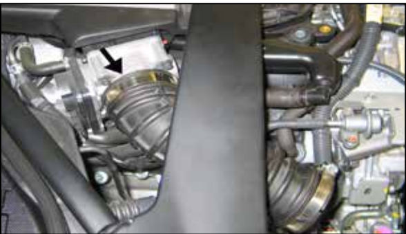
7. Loosen the hose clamp that secures the right side intake tube to the throttle body.
