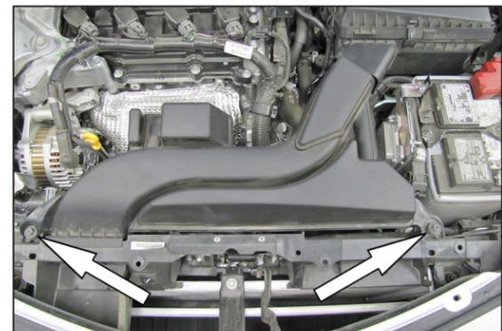
5. Remove the two bolts securing the fresh air intake to the core support and then remove the fresh air intake.
