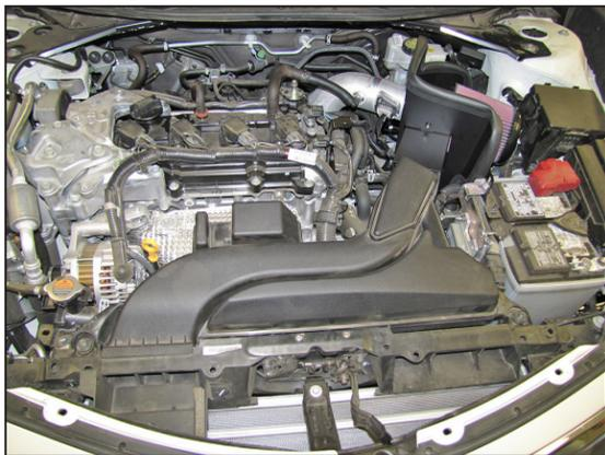
29. Install the fresh air intake scoop and secure with the factory hardware.
