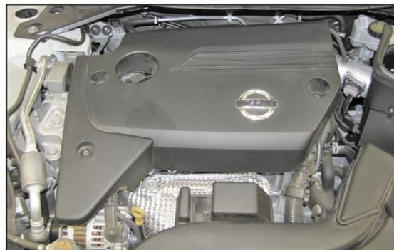
31. Install the engine cover and secure with the factory hardware.
