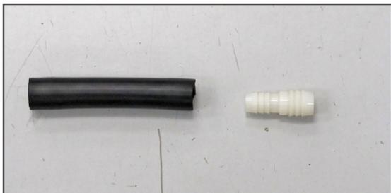
23. Install the provided hose mender into the provided crank case vent hose.
