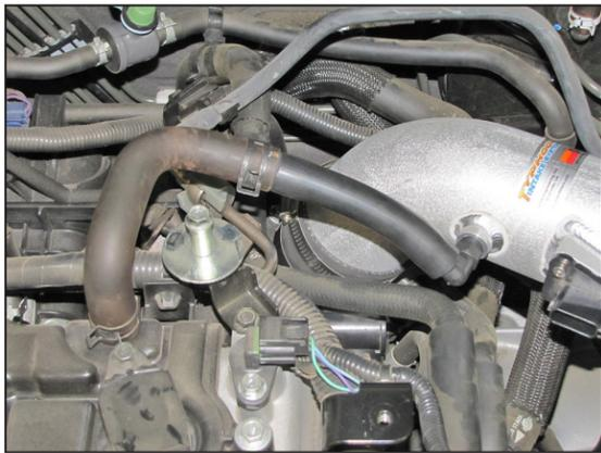
26. Connect the factory crank case vent hose to the hose mender and secure with the factory clamp.
