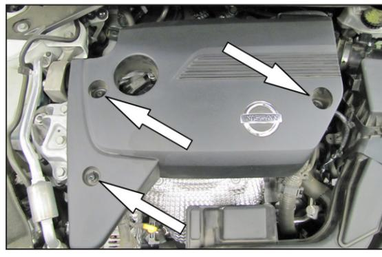
3. Remove the three bolts securing the engine cover and then lift off the engine cover.
