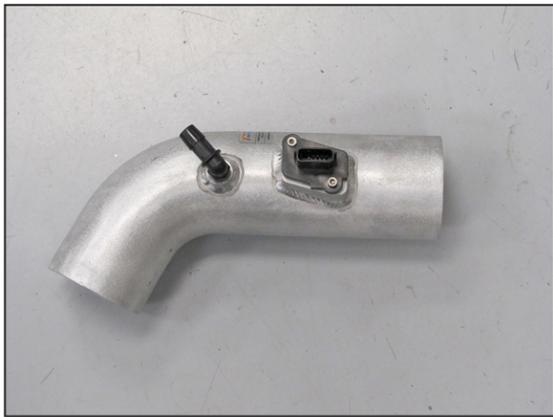
22. Install the 90° vent fitting into the K&N® intake tube as shown.
