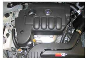
26. Reinstall the engine cover and secure with the factory bolts.
