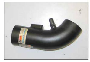
15. Install the provided 1/4"npt vent fitting into the K&N® Intake Tube as shown.
