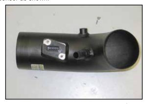
17. Install the mass air sensor into the K&N<sup>®</sup> intake tube and secure with the provided hardware.
