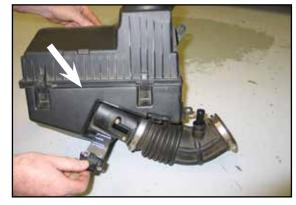
16. Remove the two bolts which secure the mass sensor to the intake tube and remove the mass air sensor as shown.
