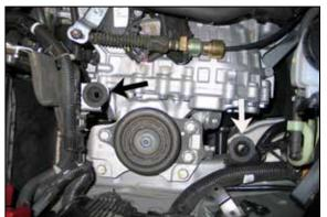
9. Remove the two rubber air box mounting grommets shown.
