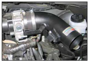
18. Install the K&N® intake tube into the silicone hose at the throttle body and align with the mounting bracket. Secure with the provided hardware and hose clamp.
