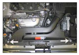
4. Remove the two bolts that secure the fresh air inlet assembly.
