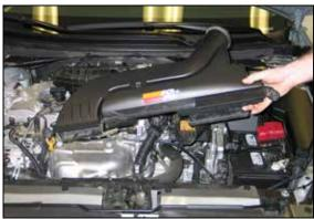
5. Remove the fresh air inlet assembly from the air box and radiator core support.
