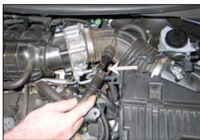
6. Release crank case vent hose spring clamp and then disconnect the crank case vent hose from the intake tube.
