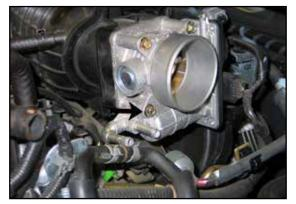
12. Remove the lower-front throttle body mounting
