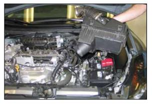
8. Remove the air box assembly from the vehicle. NOTE: K&N Engineering, Inc., recommends that customers do not discard factory air intake.
