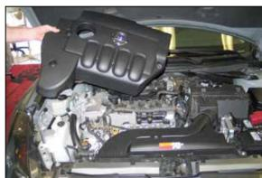
3. Remove three bolts which secure the engine cover and then remove the engine cover.
