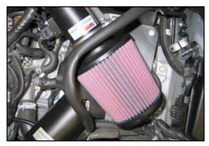
25. Install the K&N® air filter onto the K&N® intake tube and secure with the provided hose clamp. NOTE: Drycharger® air filter wrap; part # RU-4990DK is available to purchase separately. To learn more about Drycharger® filter wraps or look up color availability please visit http://www.knfilters.com®.
