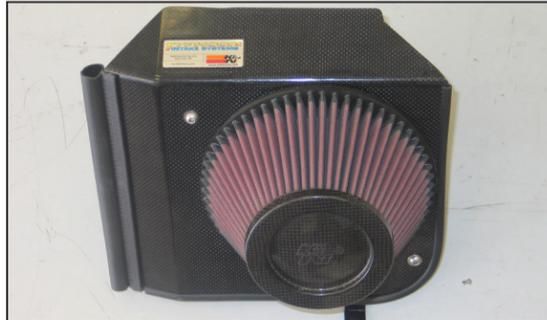
17. Install the K&N® air filter onto the filter adapter and secure with the provided hardware.
