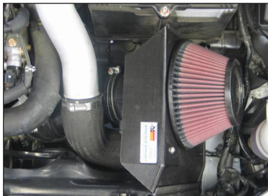
19. Install the mass air sensor/filter assembly into the into the factory intake tube and secure with the factory hose clamp.
