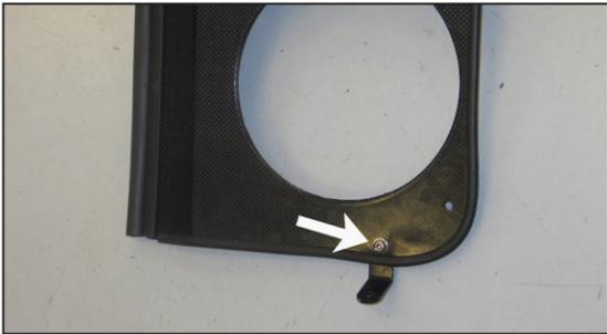
11. Install the provided heat shield mounting bracket (070102) onto the heat shield using the provided hardware.
