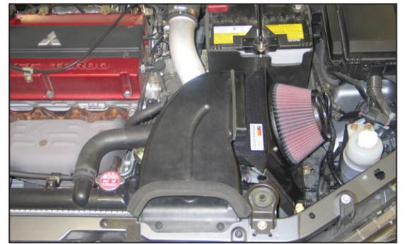
22. Clip the fresh air supply duct onto the heat shield and secure the front with the factory plastic screw.
