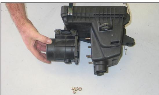
14. Remove the four mass air sensor mounting bolts; then remove the mass air sensor as shown.
