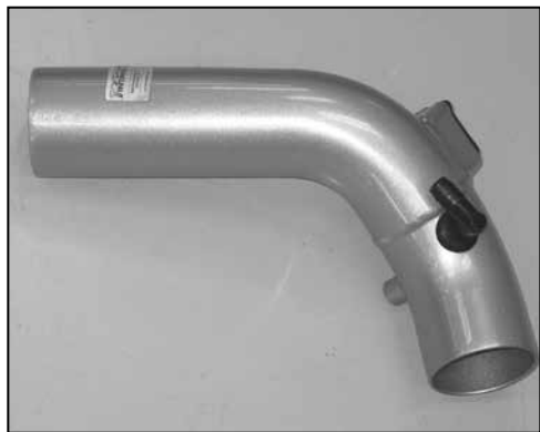
23. Install the 90° barbed fitting into the grommet that was installed into the K&N® intake tube in the previous step.
