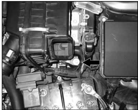
8. Remove the bolt shown that secures the air filter assembly to the mounting bracket.
