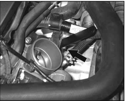
18. On vehicles equipped with an EGR tube, unhook the engine wiring harness from the clip and move the wiring harness rearward as shown. Install the intake tube mounting bracket (06724) onto the intake manifold and secure with the provided hardware.
