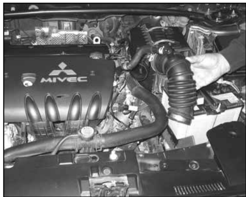
7. Remove the stock intake tube from the vehicle as shown.
