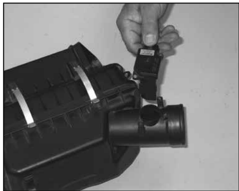
20. Remove the two screws that secure the mass air sensor into the factory air box and remove the mass air sensor as shown.
