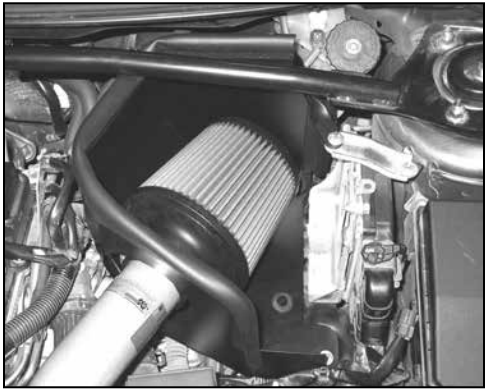
26. Install the K&N® air filter onto the intake tube and secure with the provided hose clamp.
