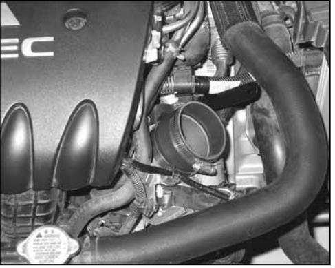
19. Install the provided silicone hose (08284) onto the throttle body and secure with the provided hose clamps. NOTE: On vehicles equipped with a 2.4L engine with the larger throttle body, use the supplied silicone hose #084016.
