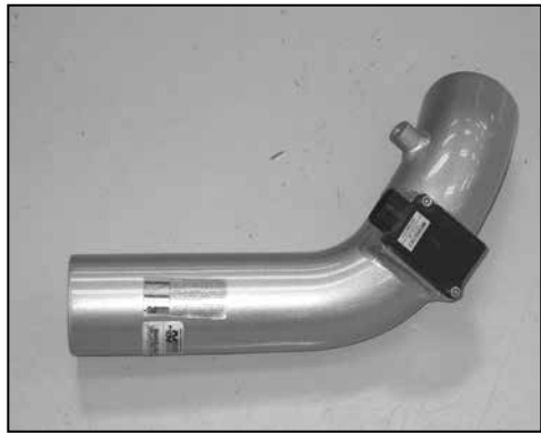
21. Install the mass air sensor into the intake tube and secure with provided hardware.
