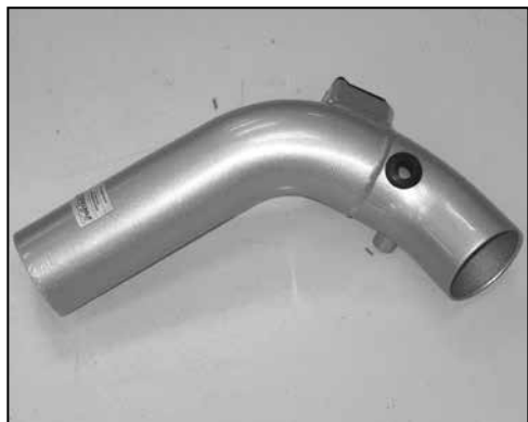
22. Install the provided 1/2" ID grommet (08064) into the intake tube as shown.
