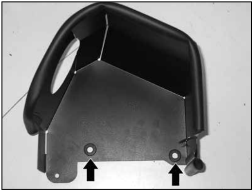
13. Install the two 7/16" ID grommets (08092) that are provided into the mounting holes in the heat shield as shown.
