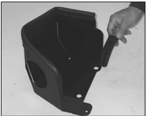
12. Install the short piece of the edge trim onto the heat shield as shown. NOTE: Some trimming of the edge trim may be needed.
