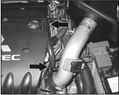
25. Install the provided crank case vent hose onto the 90° barbed fitting on the K&N® intake tube. Then attach the open end of the vent hose onto the valve cover vent port as shown.
