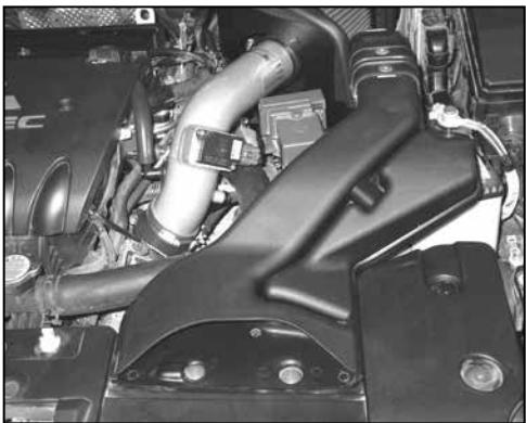
28. Reinstall the fresh air intake scoop and secure with the factory retaining clips.
