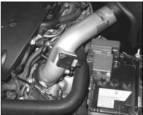
24. Install the K&N® intake tube into the silicone hose at throttle body and align with the mounting bracket installed in step #18. Secure the intake tube with the provided hose clamp and hardware. NOTE: It may be necessary to reposition the positive battery cable to obtain proper clearance of the tube.
