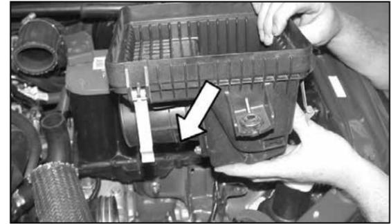
7. Remove the two bolts on the lower air cleaner assembly, then, lift up the lower assembly to unclip the mass air sensor electrical connection. Unclip the mass air sensor wire harness from the bottom the lower air cleaner assembly, then, remove the lower air cleaner assembly as shown.
