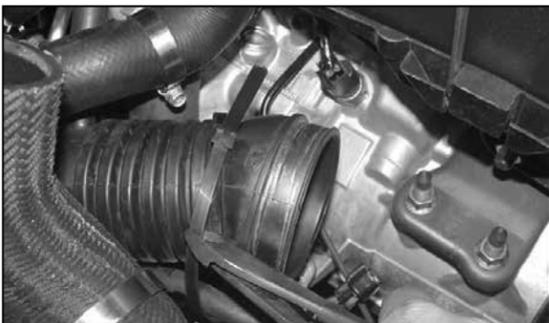
14. Using a pair of dykes, cut the clip tie that secures the vent hoses to the intake tube.
