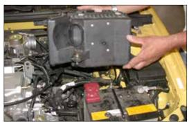
9. Pull upwards to remove the air cleaner assembly as shown.
