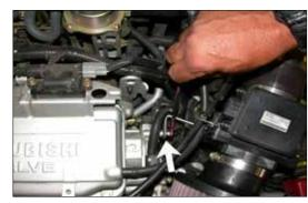
22. Tighten the hex bolt on the bracket at the threaded boss on the cam cover, adjust for best fit and clearance and adjust if necessary.
