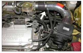
17. Install the provided silicone hose onto the cam cover and onto the intake tube as shown.
