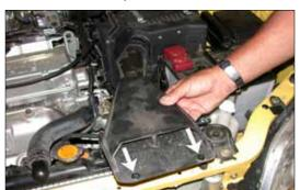
4. Depress the center pins to release the push clips from the radiator core support, then remove the air inlet duct as shown.
