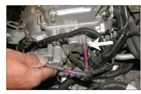
11. Remove the hex bolt on the threaded boss on the head as shown.
