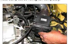
16. Secure the bracket on the mass air sensor assembly to the threaded boss from step 11 using the stock hex bolt from the same step. Do not tighten completely.
