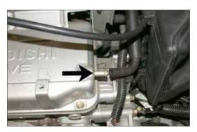
5. Remove the crank case vent hose from the cam cover as shown.
