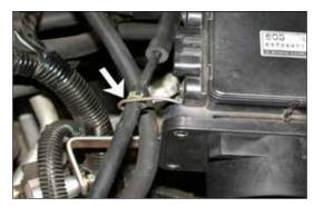
18. Slide the throttle cable into the wire hanger on the mass air sensor assembly as shown.
