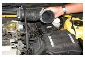
6. Loosen the hose clamps at the mass air sensor and at the throttle body, then, remove the stock intake tube as shown.
