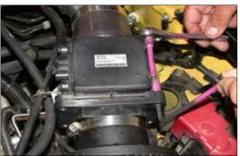
21. Tighten all the hardware on the mass air sensor assembly at this time as shown.
