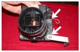
14. Assemble the mass air adapter, stock gasket, bracket, throttle cable hanger, and the stock mass air sensor using the provided hardware as shown. Do not completely tighten the hardware at this time. NOTE: The two longer cap screws are located on the side shown. (See arrows)
