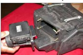
10. Remove the four hex nuts that secure the mass air sensor to the air cleaner assembly, then, remove the mass air sensor as shown.
