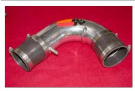
12. Install the silicone hoses and hose clamps onto the intake tube as shown, but do not tighten completely.
