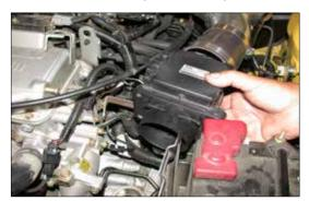
15. Slide the mass air sensor assembly into the silicone hose on the intake tube as shown. Snug the hose clamp but do not tighten completely.
