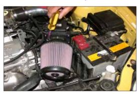
19. Install the K&N® air filter onto the mass air adapter and secure with the provided hose clamp as shown.
