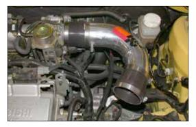
13. Install the intake tube onto the throttle body, but do not tighten completely at this time.
