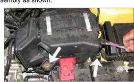
8. Loosen the two hex bolts on the air cleaner assembly as shown.
