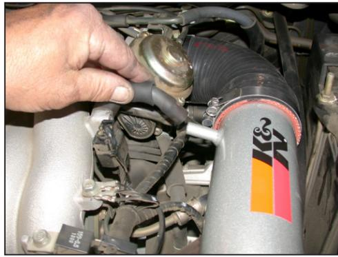
32. Reconnect the crankcase vent hose to the vent on the intake tube as shown.
