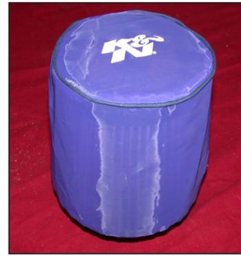
22. Install the Drycharger® onto the K&N® air filter as shown.
