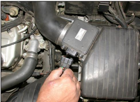
2. Disconnect the mass air sensor electrical connection as shown.
