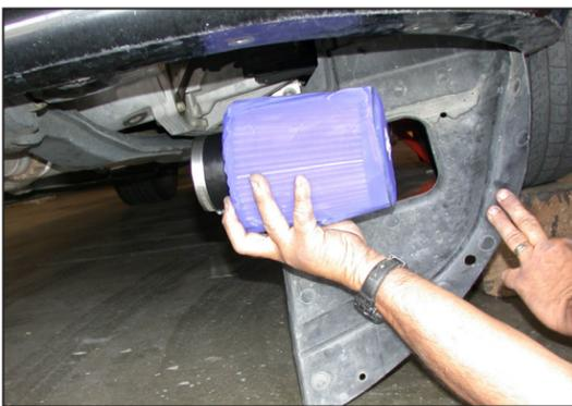
29. From underneath the vehicle install the K&N® air filter and secure with the provided hose clamp.
