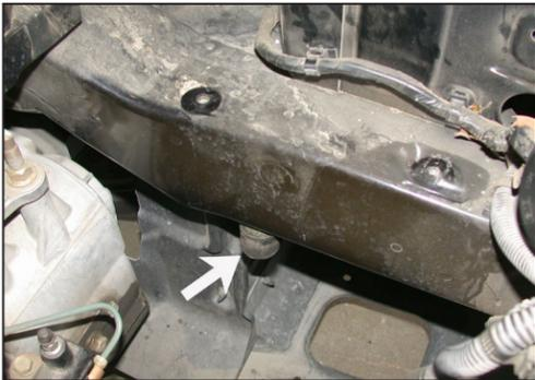
12. Install the provided rubber mounted stud into the threaded hole from step 11.
