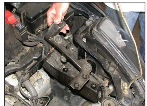
10. Remove the stock air cleaner mounting bracket as shown.
