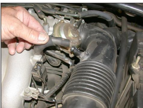
4. Disconnect the crankcase vent hose from the stock intake tube as shown.
