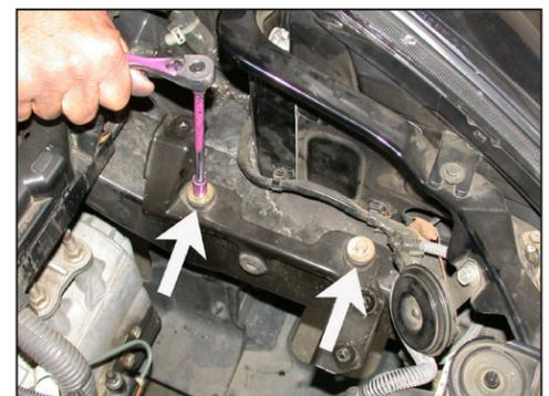
9. Remove the two bolts that secure the stock air cleaner mounting bracket as shown.
