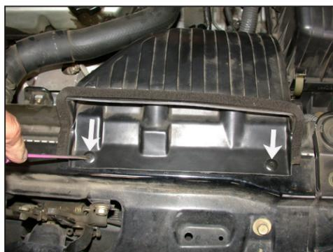
6. Depress the center pins to release the push clips on the stock air inlet duct as shown.
