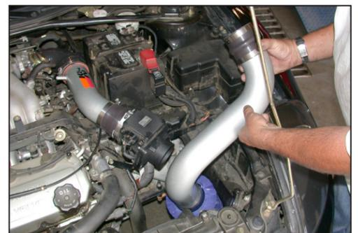
24. On manual transmission vehicles install the cold air intake tube assembly into the vehicle as shown.
