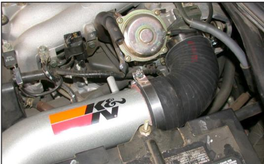
14. Slide the intake tube assembly onto the throttle body as shown but do not tighten.
