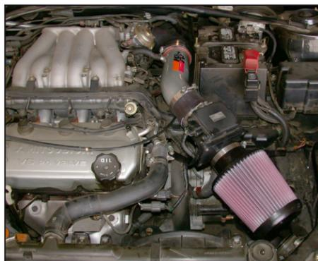
35. This K&N® high flow intake system has been designed to be used in two different configurations. In the case of inclement weather, the cold air tube can be removed and the air filter can be clamped onto the intake tube located in the engine compartment to avoid the possibility of ingesting water into the engine.
