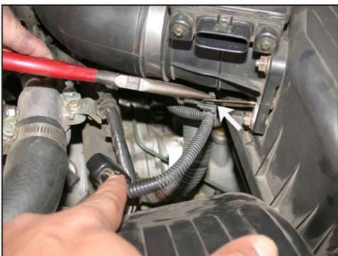
3. Unclip the mass air sensor wire harness from the stock hanger as shown.
