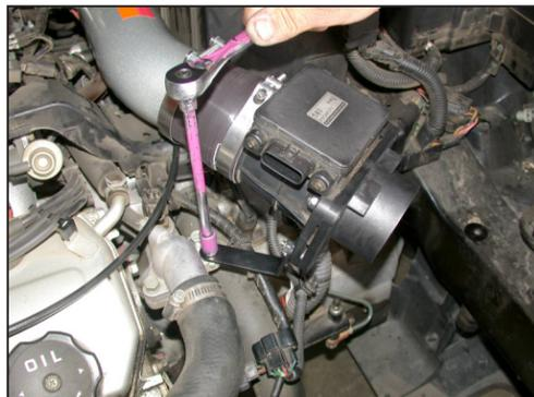
20. Secure the bracket to the water neck using the bolt removed in step 18.
