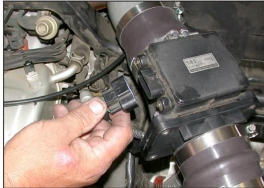
33. Reconnect the mass air sensor electrical connection as shown.
