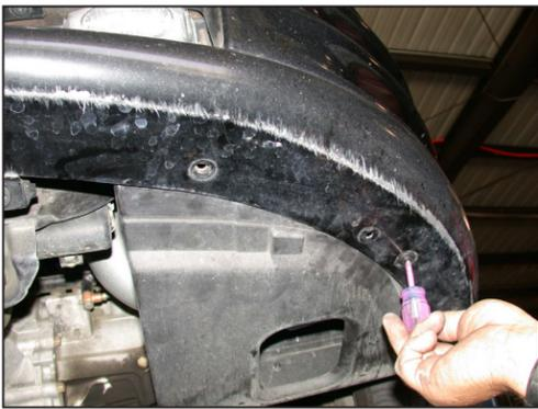
30. Reverse the removal process and re-secure the lower valance as shown.
