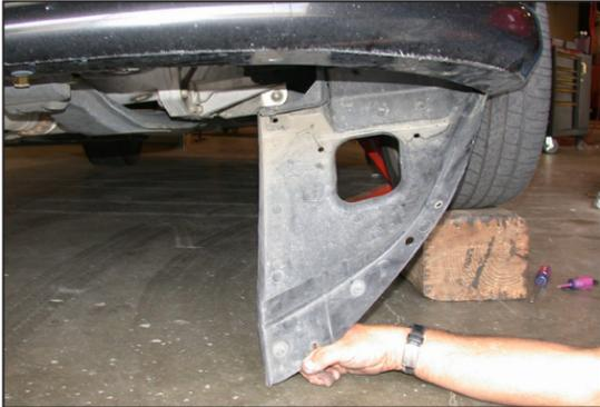
28. On automatic transmission vehicles raise the vehicle up and secure it with jack stands. Now remove the 5 screws that secure the lower valance and pull the valance back as shown.
