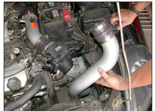
25. On automatic transmission vehicles install the cold air intake tube only as the air filter will be installed from underneath the vehicle.
