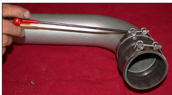
21. Install the silicone hump hose and hose clamps onto the cold air intake tube and tighten as shown.
