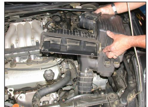
8. Remove the complete air cleaner assembly as shown.
