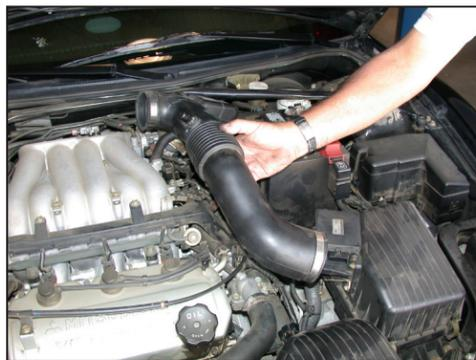
5. Loosen the hose clamps at the throttle body and at the mass air sensor, then, remove the stock intake tube as shown.
