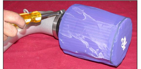
23. On manual transmission vehicles install the K&N® air filter onto the cold air intake tube and tighten as shown.
