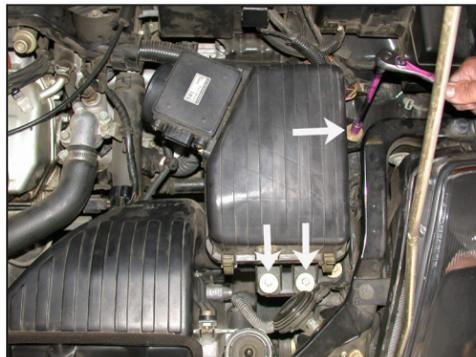
7. Loosen the 3 bolts that secure the air cleaner assembly as shown.
