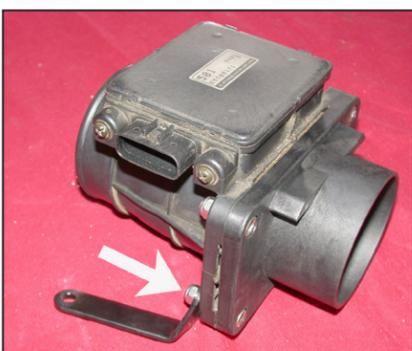
16. Assemble the provided mass air sensor adapter, bracket and the stock mass air sensor and stock gasket using the provided hardware as shown.
