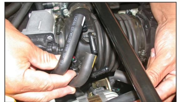
7. Disconnect the three hoses from the stock intake tube as shown.
