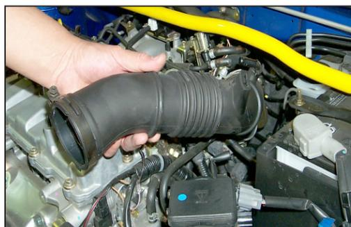
5. Loosen the hose clamps at the throttle body and at the mass air sensor, then, remove the rubber intake hose.
