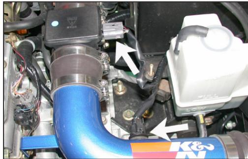
37. Reconnect the mass air sensor, and air temperature sensor electrical connections.
