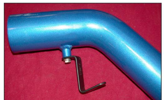
27. Install the "Z" bracket onto the threaded boss on the K&N® cold air intake tube and secure with the provided hardware.
