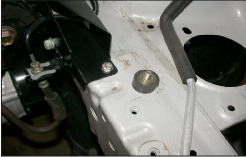
29. Install the rubber mounted stud into the threaded hole on the inner frame rail as shown.
