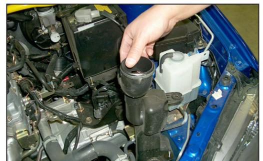
8. Loosen and remove the secondary air inlet duct that attaches to the air cleaner assembly and remove.
