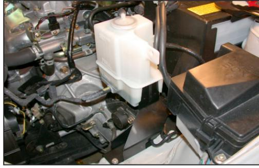
16. Slide the coolant reservoir onto the new support bracket as shown.
