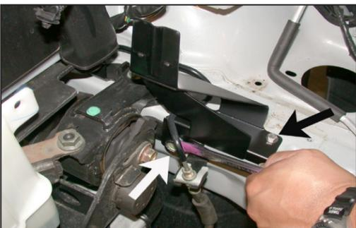
15. Install the new coolant reservoir support bracket using the bolt removed in step 14, then, secure it with the provided hardware as shown.
