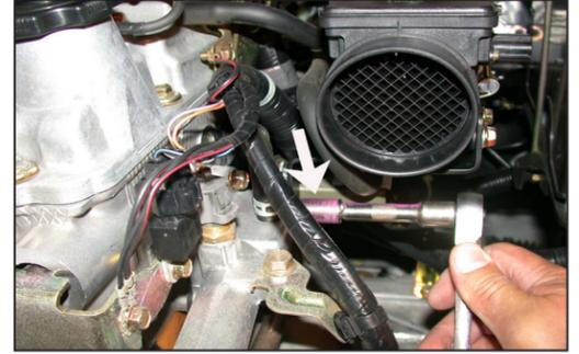
23. Secure the mass air bracket to the original fuel line support bracket using the bolt removed in step 20.
