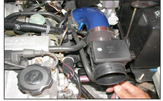
22. Slide the K&N® throttle body tube into the silicone hose on the throttle body, but do not tighten at this time.
