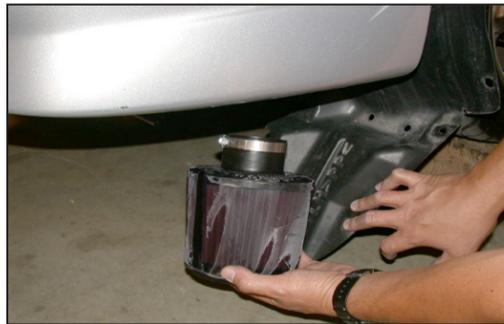
35. From underneath the vehicle install the K&N air filter onto the K&N cold air intake tube and secure with the provided hose clamp.
