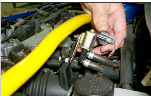
3. Remove the purge control valve from the stock rubber intake tube.
