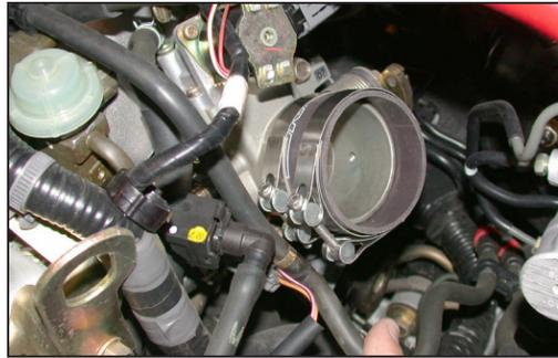
17. Install the provided silicone hose onto the throttle body and secure with the provided hose clamp.
