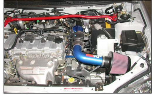
39. This K&N high flow intake system has been designed to be used in two different configurations. In the case of inclement weather, the cold air tube can be removed and the air filter can be clamped onto the intake tube located in the engine compartment to avoid the possibility of ingesting water into the engine.
