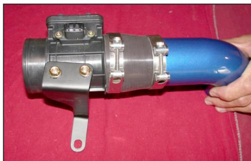
21. Secure the provided "Z" bracket to the mass air sensor using the provided washers and the original mass air bolts from step 12.
