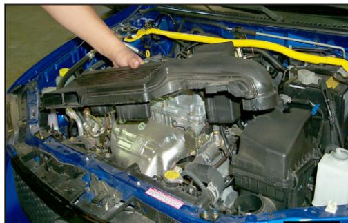
6. Loosen and remove the two nuts that secure the air inlet ducting to the top of the radiator core, then, remove the air inlet ducting.
