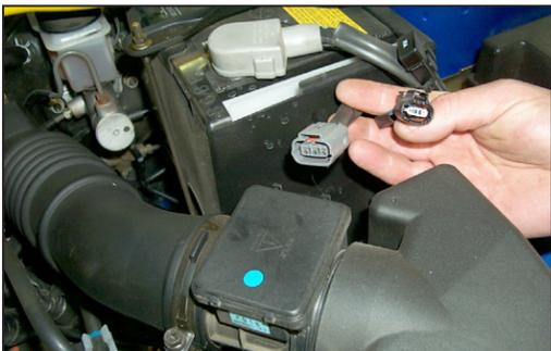
2. Disconnect the mass air sensor and air temperature sensor electrical connections.
