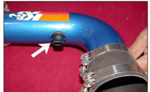
25. Install the provided grommet into the hole on the K&N® "L" tube, then, install the air temperature sensor into the grommet.
