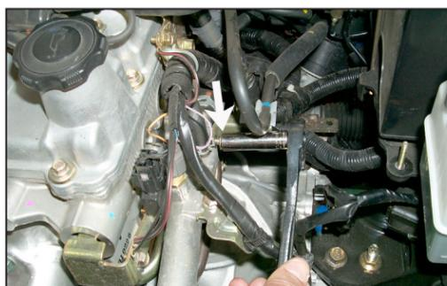
20. Remove the bolt that secures the fuel line support bracket as shown.
