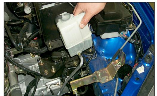
9. Slide the coolant reservoir upwards to release the reservoir from the support bracket as shown.
