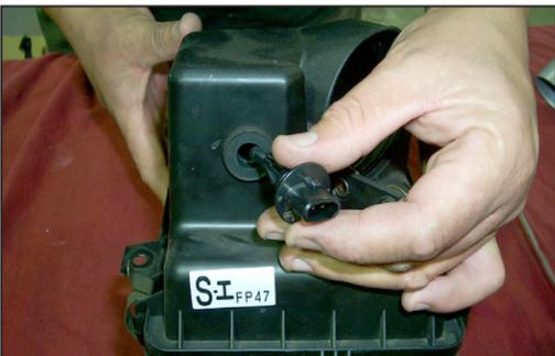
13. Remove the air temperature sensor from the air cleaner lid as shown.
