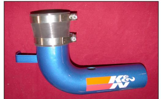
24. Install the remaining step hose and hose clamps onto the K&N® intake tube but do not tighten completely.
