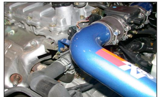
26. Slide the K&N® "L" tube onto the mass air sensor and line up the tube bracket with the ground bracket and secure with the stock bolt.
