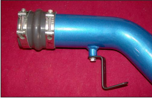
28. Install the silicone hump hose onto the cold air intake tube and secure with the provided hose clamp.
