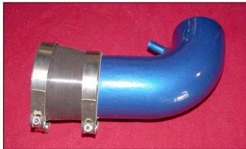
18. Install the silicone step hose onto the throttle body tube and secure with the provided hose clamp, but do not tighten completely.
