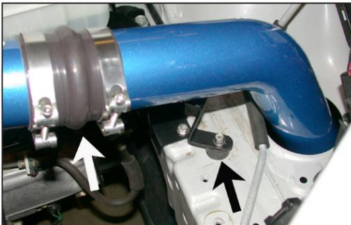
30. Install the cold air tube into the hole in the inner fender then slide the silicone hose onto the short "L" tube as shown and secure with the provide hose clamp. Also secure the "Z" bracket to the rubber mounted stud with the provided washer and nylock nut.
