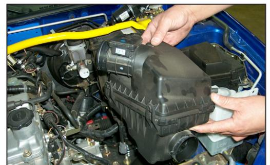
7. Loosen and remove the nut and bolt that secure the air cleaner assembly, then, remove the air cleaner assembly.
