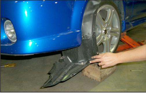
11. Jack the vehicle up and support it with jack stands, then, remove the inner fender wheel house valance as shown.
