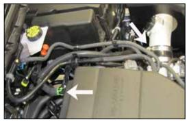
22. Install the short length of the crankcase vent hose onto the valve cover port and then attach the open end to the fitting installed into the K&N<sup>®</sup> intake tube.
