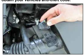
2. Disconnect the mass air sensor electrical connection and then unhook the harness from the airbox mounting location.
