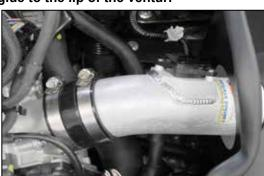
20. Install the K&N® intake tube assembly into the silicone hose at the throttle body and align with the tube mounting bracket and then secure with the provided hardware and hose clamps.
