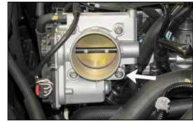
9. Remove the lower rear throttle body mounting bolt shown.
