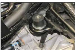
12. Install the provided rubber mounted stud onto the airbox mounting bracket using the provided hardware as shown.
