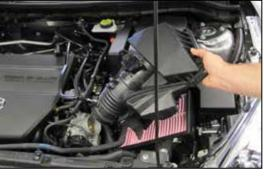
5. Remove the upper airbox assembly from the vehicle as shown.
