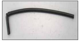
21. Assemble the crankcase vent hoses and 90° barbed fitting as shown.
