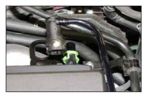
4. Unhook the crankcase vent line from the valve cover port as shown.
