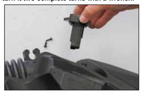
17. Remove the two screws which secure the mass air sensor into the factory airbox and then remove the mass air sensor as shown.
