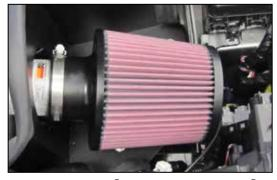
23. Install the K&N® air filter onto the K&N® intake tube and secure with the provided hose clamp.
