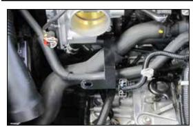
10. Install the tube mounting bracket (083137) onto the throttle body and secure with the factory bolt removed in step #9.
