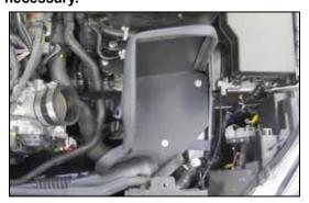
15. Set the heat shield into position on the rubber mounted stud, and then secure the heat shield with the provided hardware.
