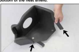
14. Install the edge trim onto the heat shield as shown.
