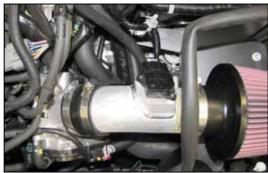
24. Reconnect the mass air sensor electrical connection.
