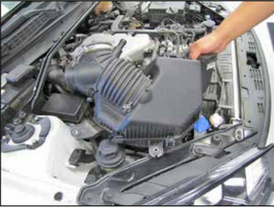
7. Lift up and remove the air box from the vehicle.
