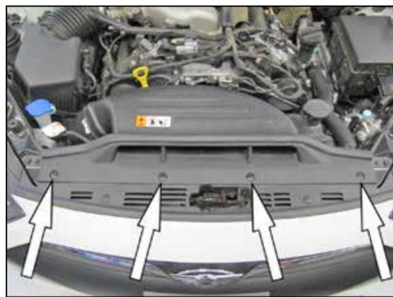
3. Remove the four plastic screws that secure the fresh air inlet scoop and then remove the scoop from the vehicle.
