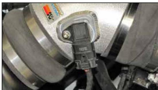
32. Reconnect the air sensor electrical connection.
