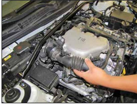
12. Remove the engine sound drum assembly from the vehicle.
