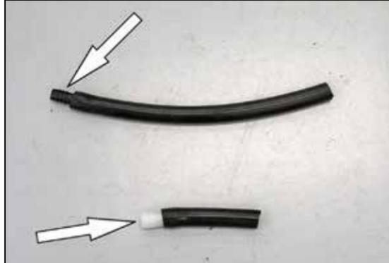
29. Install the provided hose menders into the cut sections of breather hose as shown. The 1/2" hose mender will go into the 11" breather hose. The 1/2" to 5/8" hose mender will go in the 4.5" breather hose.
