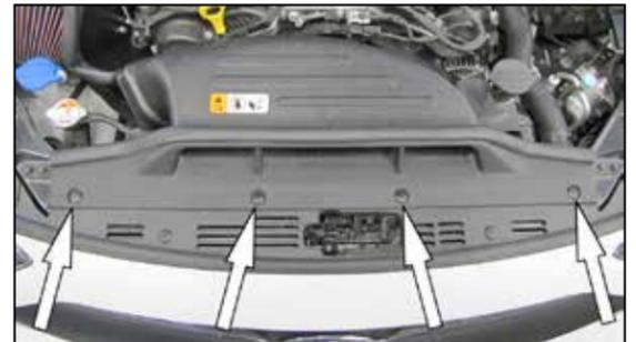
33. Reinstall the fresh air intake scoop and secure with the factory hardware.
