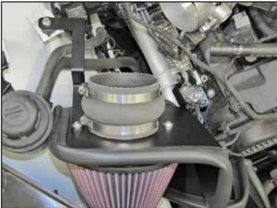
25. Install the hump hose (08418) onto the filter adapter as shown using the provided hose clamp.
