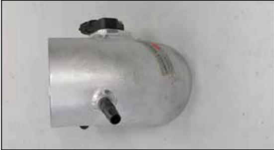
24. Install the straight vent fitting into the K&N® intake tube as shown.
