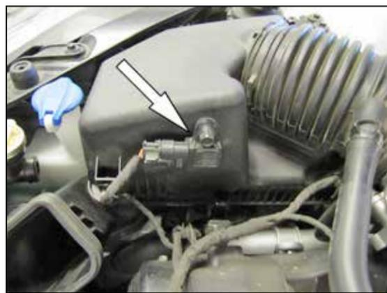
4. Disconnect the electrical connection from the inlet air sensor and unhook the wiring harness from the air box.
