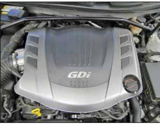
2. Lift up and remove the engine cover from the engine.
