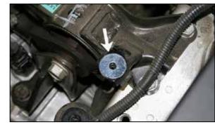
22. Place the rubber washer and fender washer onto the stock airbox mounting hole on the transmission mount as shown.
