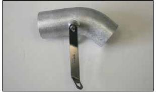
16. Install the provided "C" bracket onto the intake tube and secure it with the provided hardware.
