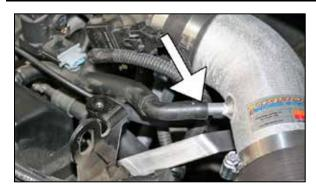
28. Install the crankcase vent hose onto the intake tube.
