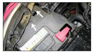
11. Remove the three screw style clips and one bolt that secure the battery cover.
