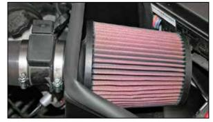
26. Attach the air filter onto the mass air flow sensor, ensuring the air filter hose clamp is installed from behind the heat shield, closest to mass air flow sensor.
