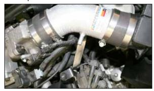
24. Install the intake tube onto the throttle body silicone hose and align the bracket with the bolt hole exposed in step #15. Reinstall the bolt removed in step #15, but do not completely tighten at this time.
