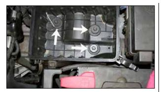
10. Loosen the three bolts that secure the lower airbox to the vehicle.
