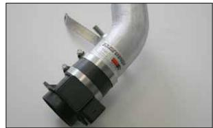
17. Install the mass air sensor onto the the intake tube with the silicone hose and two hose clamps. Tighten the hose clamps at this time.
