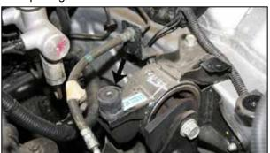
21. Install the 1" rubber mounted stud (02033) onto the stock airbox mounting hole, the mounting hole located closest to the engine.
