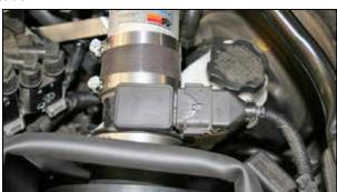
29. Reconnect the mass air flow sensor electrical connection.
