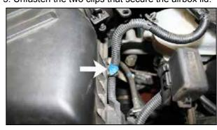
6. Unclip the mass air sensor electrical harness from airbox.
