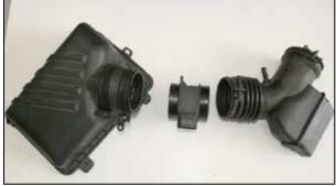
14. Separate the factory mass air flow sensor from the airbox lid and factory tube by loosening the two clamps.
