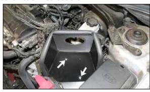
23. Install the heat shield, aligning the rear mounting hole with rubber mounted stud installed in step #21. Align the 2nd mounting hole with the mounting location the fender washers were placed in during step #22. Secure the heat shield in place with the provided hardware.
