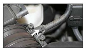
4. Unclip the mass air sensor electrical harness from the factory intake tube.
