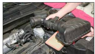
9. Remove the factory intake tube and the airbox lid from the vehicle.
