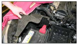
12. Remove the battery cover as shown.
