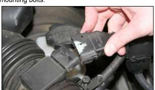
3. Unclip the mass air sensor electrical connection as shown.
