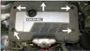
2. Remove the engine cover by loosening the 5 mounting bolts.
