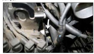
15. Remove the engine hoist bracket bolt and set aside, it will be reused at a later time.
