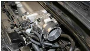
18. Install the provided silicone hose and hose clamps onto the throttle body. Secure the hose clamp on the throttle body at this time.
