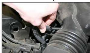
8. Disconnect the crankcase vent hose from the stock intake tube.
