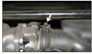
7. Loosen the hose clamp securing the factory intake tube to the throttle body.
